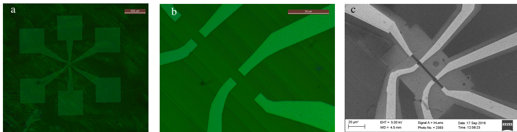
FIGURE 3.10: Fabrication process of Hall Bar on epitaxial graphene. (a) Optical image of the Bar definition and removal of graphene under pads and contacts. (b) Optical image contacts definition. (c) SEM image of the device after contacts and Pads deposition.
