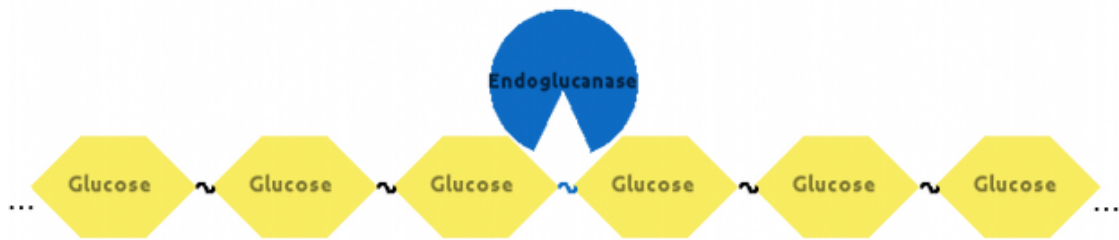
Figure 2.20: Endoglucanase enzyme type. The enzyme acts exclusively on the interior of polymer chains without differing between soluble and insoluble chains.
