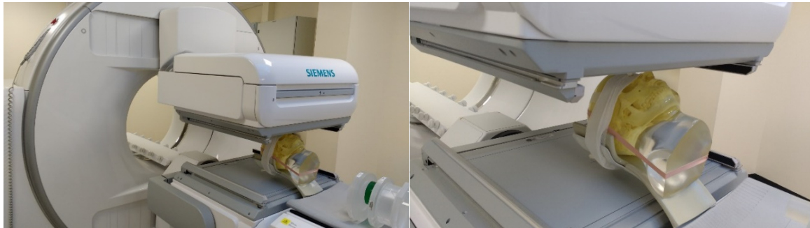
Figure 17: Striatal phantom used for FP-CIT quantification work. The images show the brain shell and assembled phantom being scanned and an example transaxial phantom image analysed in BRASS
