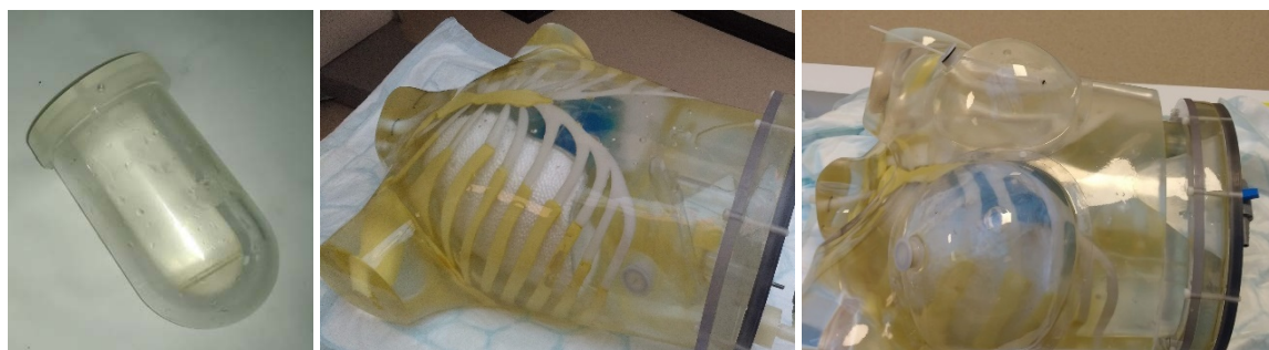
Figure 73: Anthropomorphic torso phantom (centre), with in-house replacement LV insert (left) and additional PMMA chest plate and water filled breasts (right)
