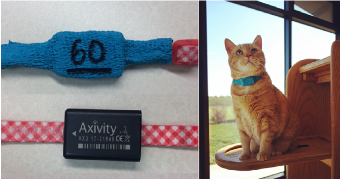
Figure 5.1: Left: AX3 sensor correctly orientated on feline collar (left bottom), and sensor labelled and secured to collar using cohesive bandage (left top). Right: Colony cat wearing sensor fitted collar.
