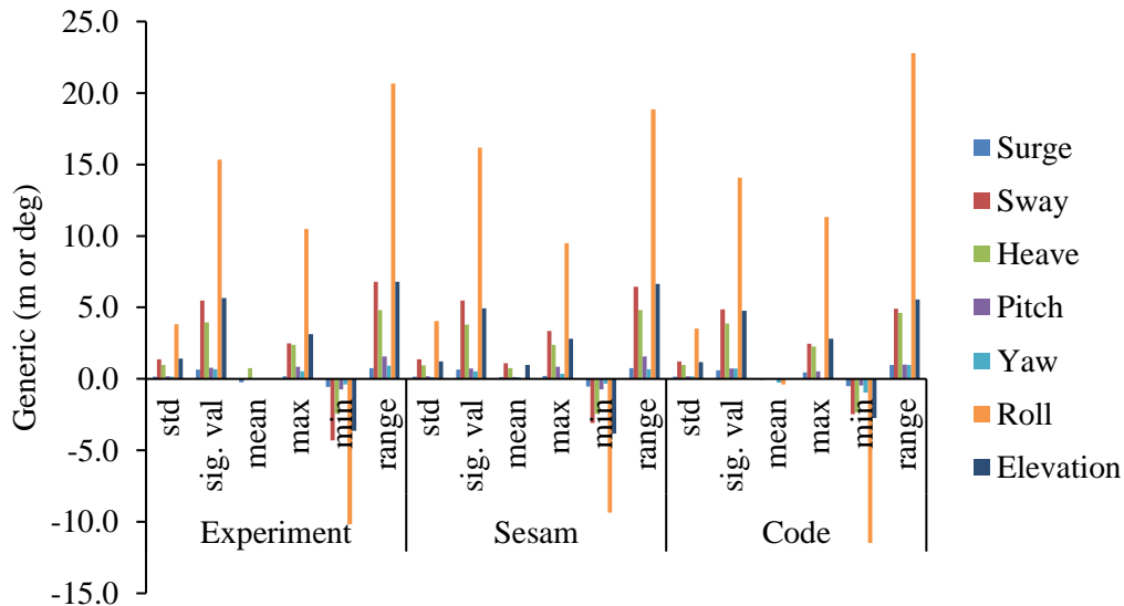
S.4 Appendix Table S2: Chart representation of Statistical Evaluation of motion amplitude time history for case a2 (T3bk1df2hs3q2)
