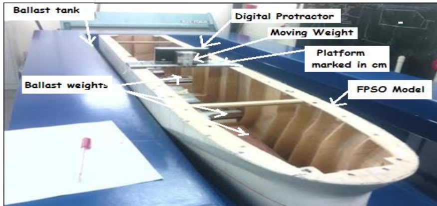
Figure 3.4 Ballast set up Newcastle University Hydrodynamic lab ballast tank.
