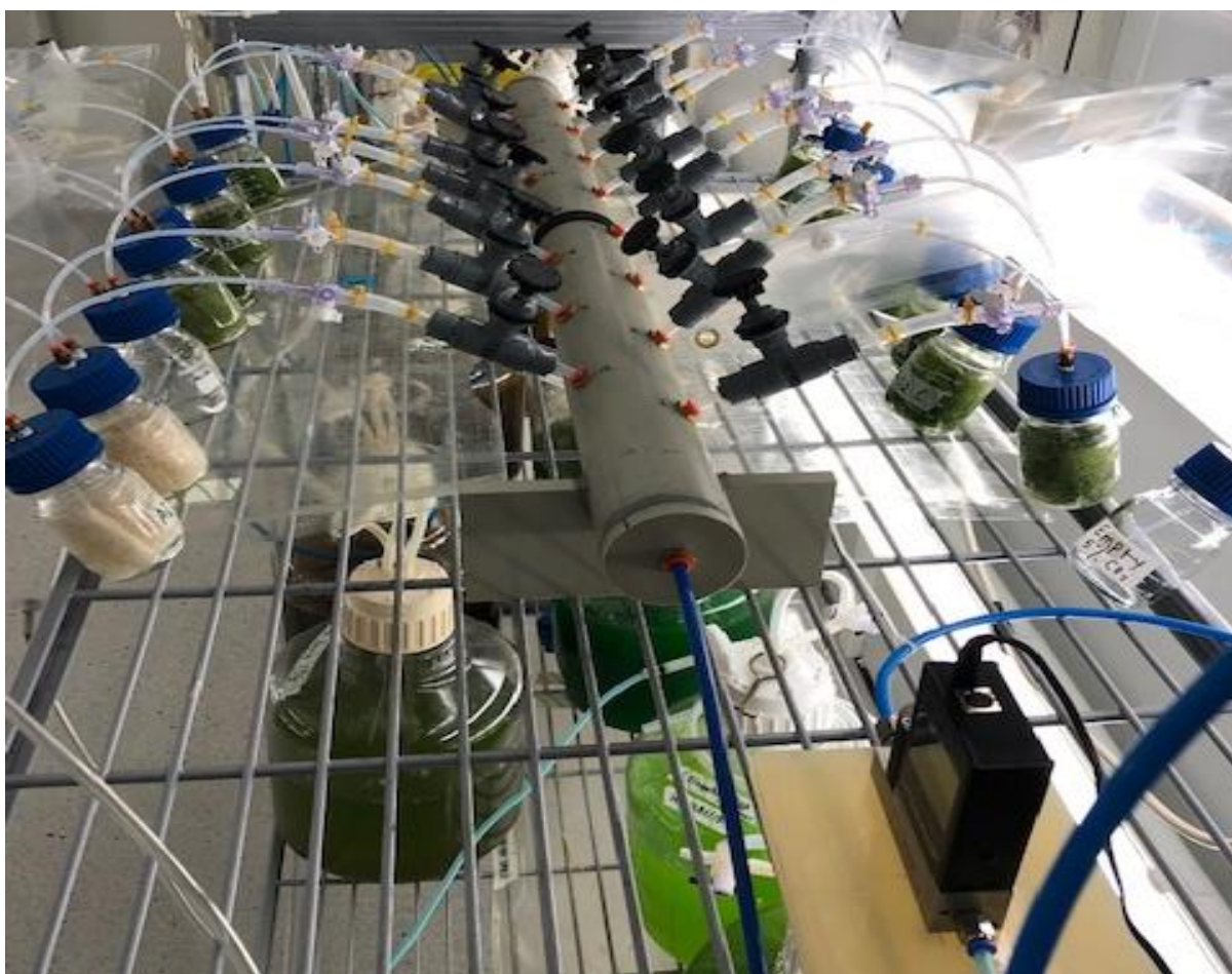
Figure 6.4: Photograph of the microalgae biocomposites rig for continuous CO 2 fixation trials. Growth condition: 18±2 °C, a 16/8 h light/dark photoperiod with 2,500 lux of illumination provided by daylight-type fluorescent lamps, and constantly aerated with 5% CO 2 , water consumption of each bioreactor bottle is approximately 1 mL day -1 , which was supplied every 72 hr via portable 1L bottle sprinkler.
