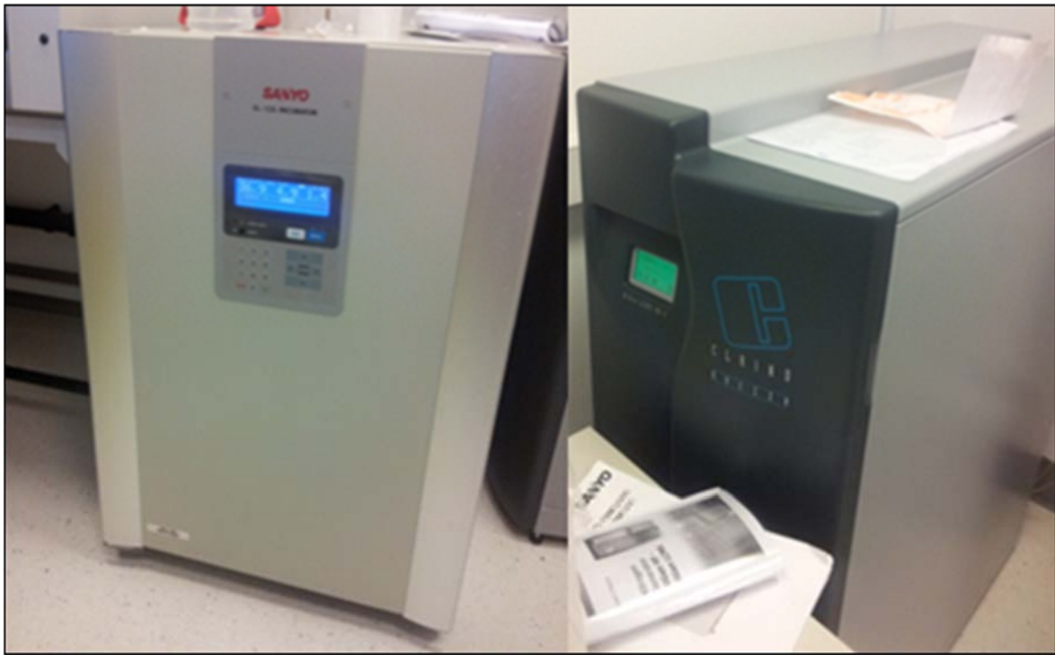
Figure 2.4 Multigas incubator for in vitro hypoxia studies (left). To maintain hypoxia, oxygen in this incubator is replaced with nitrogen delivered via a nitrogen generator (right)
