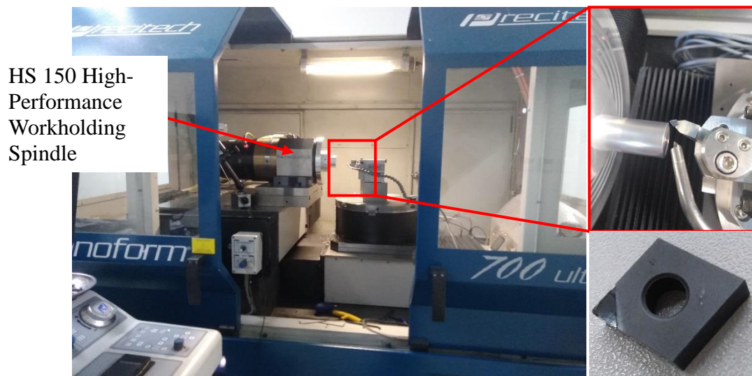
Figure 4.19 ultraprecision machine tool (Nanoform700, Precitech, USA) with PCD turning insert
