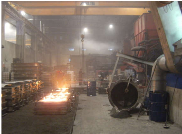
Figure 6-3: Large amounts of dusts and fumes are produced while the castings are cooling down (Photo taken by the Author)
