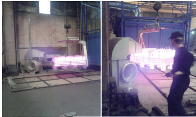
Figure 5-39: Air-quenching Facility in the Subject Plant: air-quenching fans in the plant and a batch of workpieces while being air quenched
