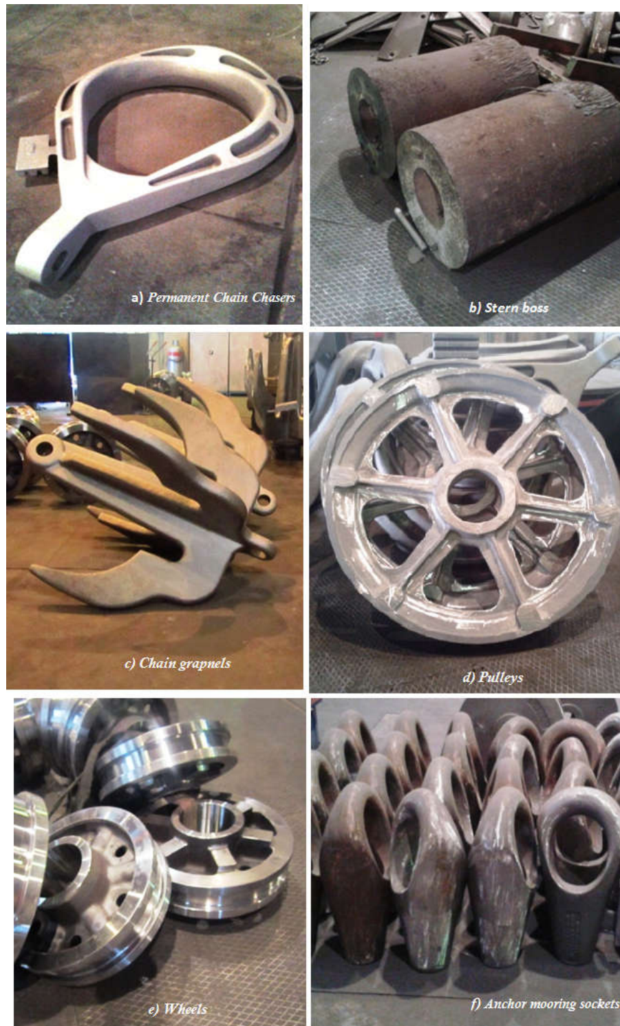
Figure 4-4: Some examples of marine & offshore products produced in the plant
