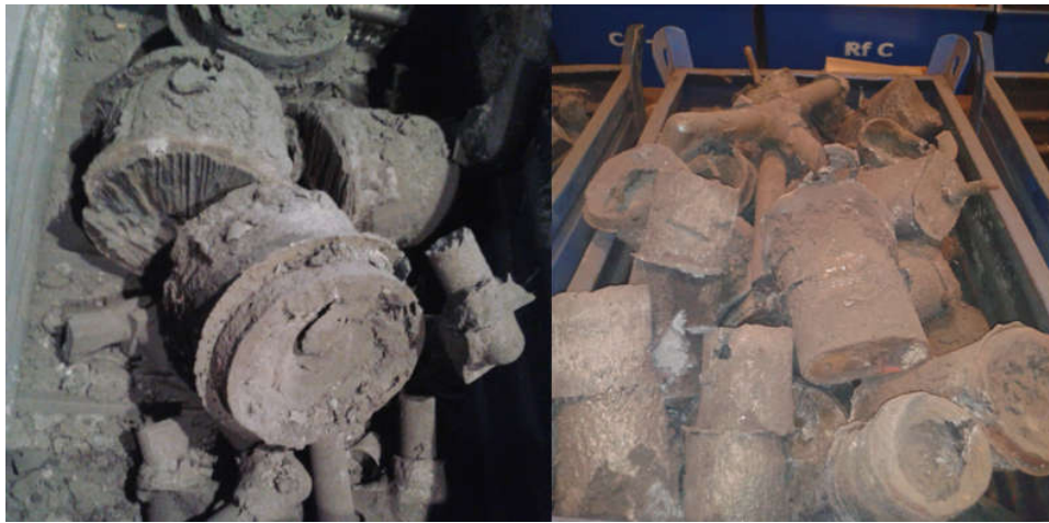
Figure 5-6: Uncleaned returns used as scrap metal in the subject plant (Photo taken by the Author)
