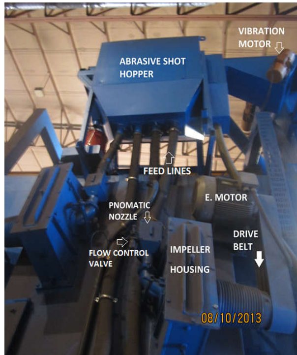
Figure G-7: Various components of the abrasive blasting system
