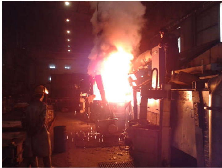
Figure 6-2: Large amounts of dusts and fumes are produced while the furnace load (i.e. molten metal) is poured to the ladles (Photo taken by the Author)
