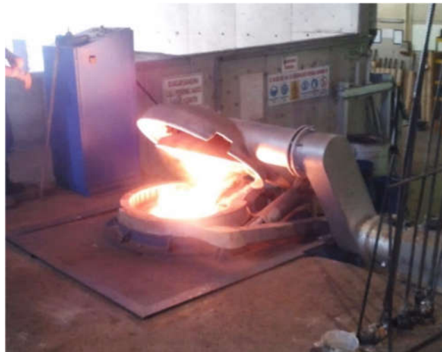
Figure 5-4: Inefficient furnace operation causing to energy losses in the subject plant (Photo taken by the Author)
