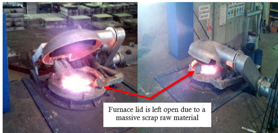
Figure 5-4: Inefficient furnace operation causing to energy losses in the subject plant (Photo taken by the Author)
