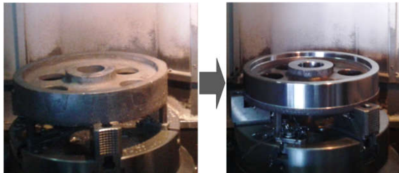
Figure 5-26: The product for case study: before (left) and after machining (right)
