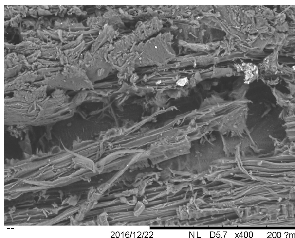
Figure 3.10 SEM image (x400) of fresh biochar catalyst (scale=200 \mu\text{m} )
