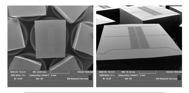
FIGURE 5.18: View of gold-coated surface biochips from the SEM internal camera. On the left, we display a overview of the 7 gold-coated specimens to observe on the rotary central platform. On the right, we show a low magnification of the entirety of a microfluidics chips at a  $55^{\circ}$  angle (chip CWqs21).
