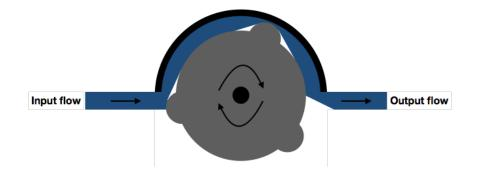
FIGURE 3.22: Schematics of a peristaltic pump. Tubing passing by the pump is compressed at specific locations, which creates a flow movement from input to output ports. The pump rotation speed is usually digitally controlled and is expressed in number of rotations per minute.
