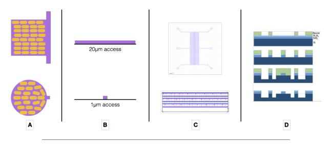
FIGURE 5.4: Considerations for the design and fabrication of microfluidics chips. (A) Top view of bacterial traps as circular or rectangular shapes in respectively channel- and surface-type chips, (B) corresponding aperture from traps to flow channels, (C) CAD design of microfeatures and (D) photolithography process overview.
