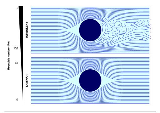
FIGURE 5.2: A reynolds number provides the ratio of inertial forces over viscosity in fluids. Fluid dynamics change and become turbulent for high reynolds numbers while low numbers are associated with an undisturbed laminar flow.
