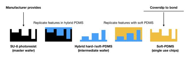
FIGURE 5.5: A master wafer is first manufactured by photolithography and contains specific microfluidics patterns to be cast onto PDMS. In order to obtain the same pattern orientation, we first generated an intermediate mould made of hybrid hard-/soft-PDMS. This intermediate was then used for the casting of final single-use biochips.
