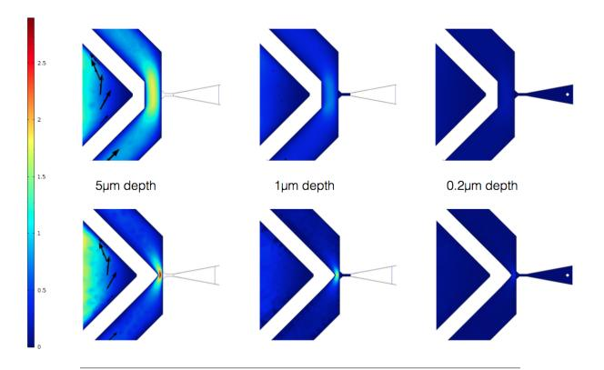
FIGURE 5.17: Models of flow acceleration towards bacterial traps in surface biochips. The three top simulation panels describe the basic flows that occur, from left to right, at  $5\mu m$ ,  $1\mu m$  and  $0.2\mu m$  depths levels in basic surface chip design. Bottom frames correspond to the same simulation results for a chip that displays higher flow near bacterial traps. The left-hand side legend displays colour-coded differential flow velocities.
