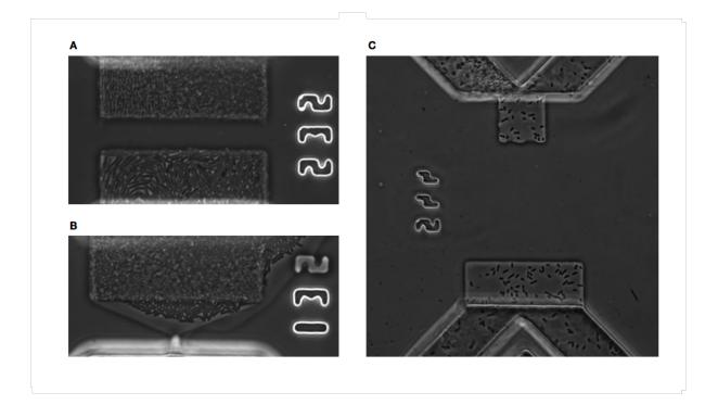
FIGURE 5.25: Potential situations following continuous bacterial growth in surface-type biochips. (A) describes an adequate bacterial growth, (B) colonisation of the diffusion surface by cells and (C) a clogging effect (top left) due to residual organic matter stuck in a flow channel.
