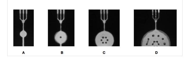
FIGURE 5.11: Fluorescence images of channel-type microfluidics features immersed in a red dye. Features visible over a black background correspond to cellular traps and diffusion channels. (A), (B), (C) and (D) respectively represent bottom traps widths of  $10\mu m$ ,  $20\mu m$ ,  $30\mu m$  and  $40\mu m$ . Top cellular channels have a width of  $1\mu m$  and diffusion channels  $0.7\mu m$  on average.
