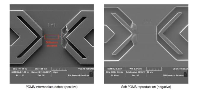
FIGURE 5.19: Potential defects in the reproduction of PDMS microstructures from silicon wafers. Left panel displays the intermediate mould that tore a microfeature, likely during separation from template. The red rectangle is placed around the diffusion channel that, despite flow channel collapse, was accurately reproduced. Right panel shows reproduction of the same defect onto soft PDMS chips.
