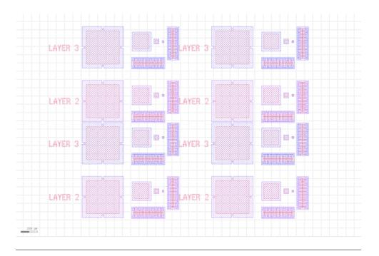
FIGURE 5.3: Redundant mask alignment pattern for the construction of multiple depths on silicon wafers. Each colour represents a specific depth layer.
