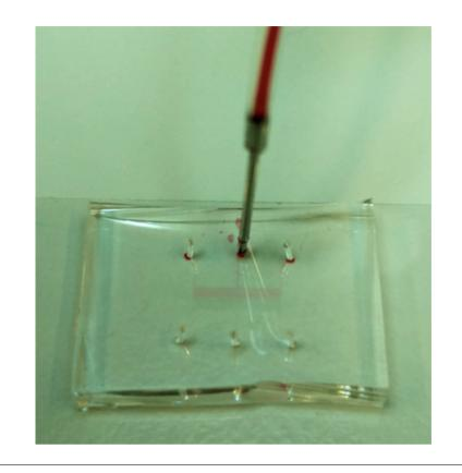
FIGURE 5.22: Flow dynamics test of a surface-type biochip with a coloured compound. Input flow from a syringe plugged into the top middle port splits symmetrically into left-/right-hand part of the microfluidics design (biological replicas). The flow is contained within the top half of the chip and separated from bottom replicas by a narrow diffusion surface.
