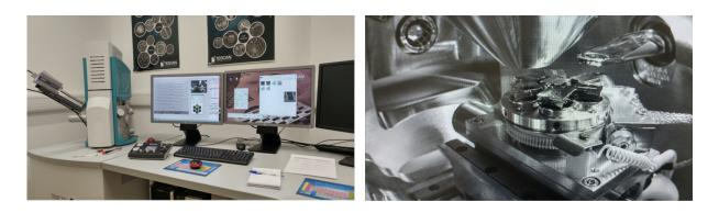
FIGURE 5.9: Overview of a scanning electron microscope. On the left, we show a picture of the microscope setup, with an incubation chamber for specimen visualisation, an electron beam apparatus and a computerised platform for dynamic treatment of data. On the right, we display the view from the interior of the specimen observation chamber. A central platform features up to 7 specimens that should be gold-coated before imaging.
