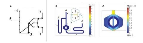
FIGURE 5.7: For a given chip design, (A) nodal analysis describes flow directions and pressure drops, (B) finite element methods provide finer fluid dynamics methodologies including (C) variable flow regimes in crosssections. Adapted from [65]
