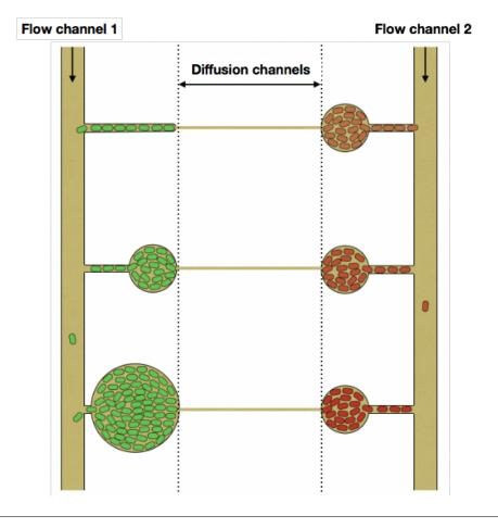
FIGURE 5.8: Simplified schematics of channel-type microfluidics biochips. Bacterial strains can be observed simultaneously in variable size microreactors connected by a thin diffusion channel. Inducers can be added to flow channels directly or propagated in diffusion channels.
