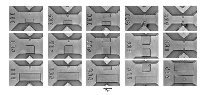
FIGURE 5.23: Microfeatures of surface biochips immersed in LB medium under an inverted microscope. Soft PDMS was bonded to a coverslip, plugged at input/output ports and observed in microscopy before applying a flow of cells.
