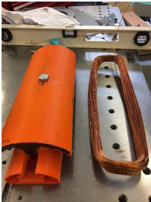
(a). Windings removed from the bobbin
