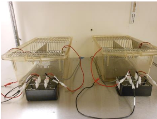
Figure 2.1: Photographs of drinking apparatus used for all experiments presented in this thesis A. View from above a single drinking chamber B. View from the side of a single drinking chamber C. Front view of two drinking chambers with med associates lickometer D. Front view of all eight drinking chambers on shelving.
