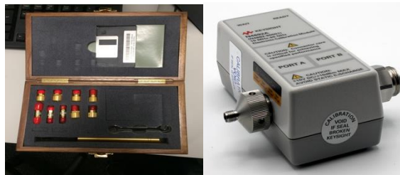
Figure 5-14. Standard mechanical and electronic calibration kits for Agilent PNA.
