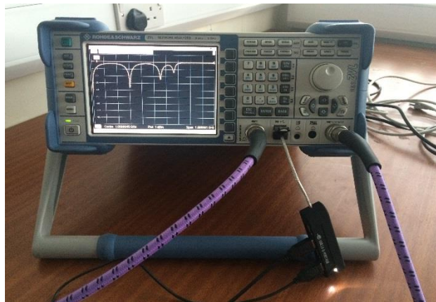
Figure 5-11. Rohde & Schwarz network analyser, frequency range from 9 kHz to 3GHz.
