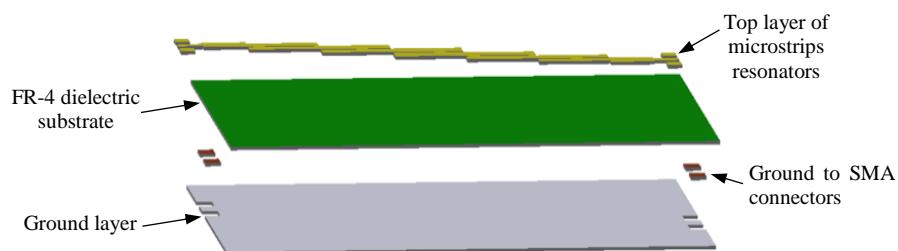
Figure 5-1. Schematic illustration of build-up PCB layers to construct microstrip filter
