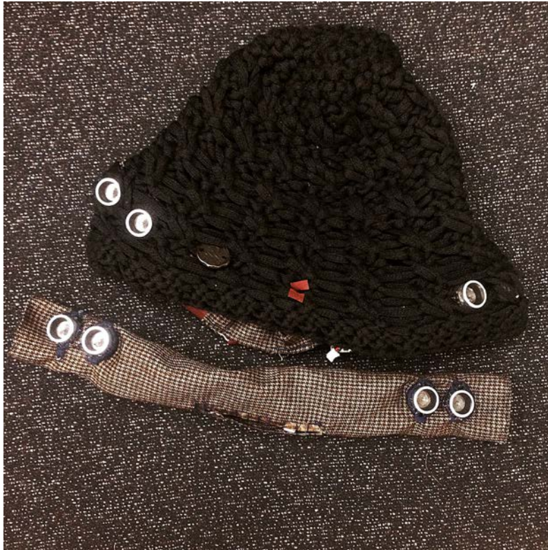
Fig. 5.3.2 The ultrasonic hat. Image: S Chen
