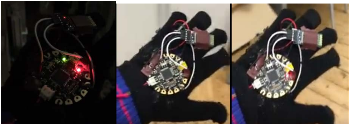
Fig 4.2.1.3 Experiment with Pulse Sensor Arduino for Heart Rate detection.
