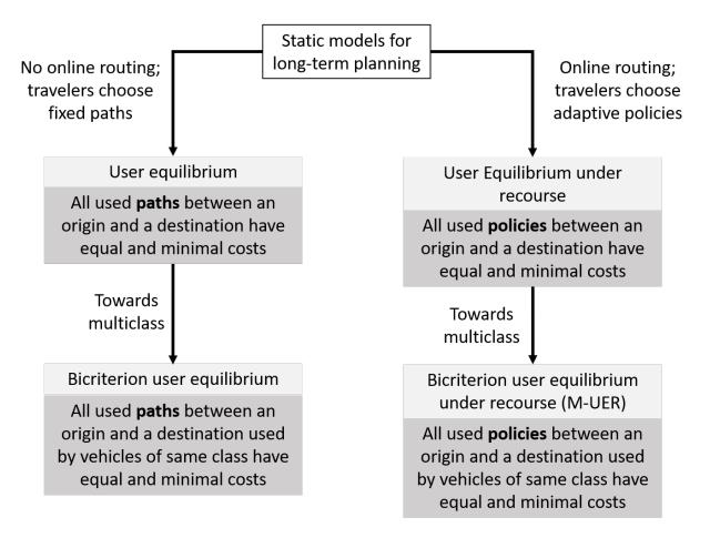
Figure 5.1: Schematic of M-UER model and its relation to other models in the literature
