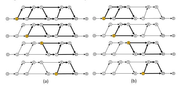
Figure 3.2: Decision routes for each highlighted diverge point using (a) the complete-route generation (CRG) approach, and (b) the sub-route generation (SRG) approach
