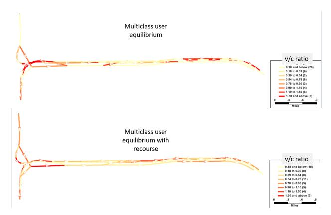
Figure 5.6: Comparison of v/c ratios between M-UER runs and runs based on multiclass traffic assignment for the NTE network
