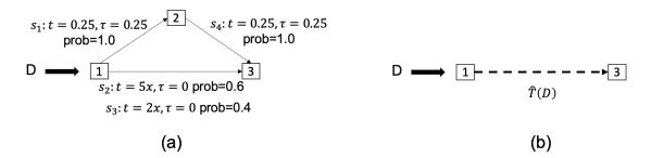
Figure 6.5: (a) Small network and (b) a contracted network with artificial link representing demand as a function of cost
