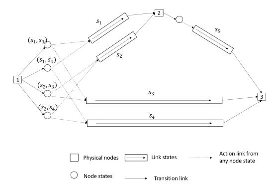
Figure 5.3: Network transformation for the network in Figure 5.2 by splitting it into node-states, link-states, and physical nodes
