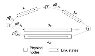
Figure 6.4: Network transformation show the node to link-state connection with probabilities on each arc expressed in terms of  $\rho$  variable.
