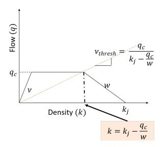
Figure 3.3: Trapezoidal fundamental diagram for modeling traffic flow
