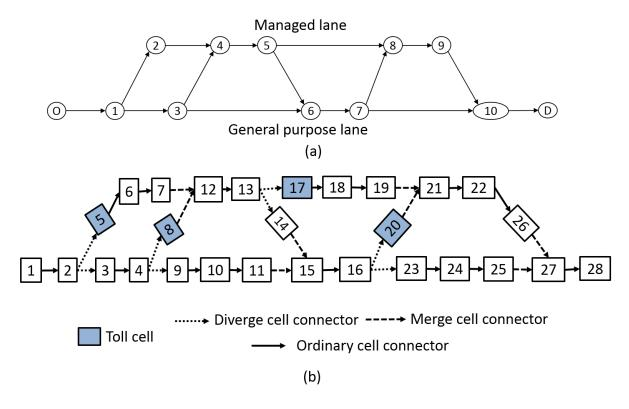
Figure 3.1: (a) Multiple entrance multiple exit managed lane network (b) Representation of the same network in cell transmission model
