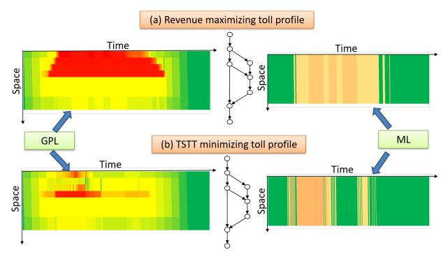
Figure 3.11: Time-space diagram showing the ratio of current density to the maximum jam-density for each cell on the GPL and the ML, for (a) revenue-maximizing toll profile, and (b) TSTT-minimizing toll profile
