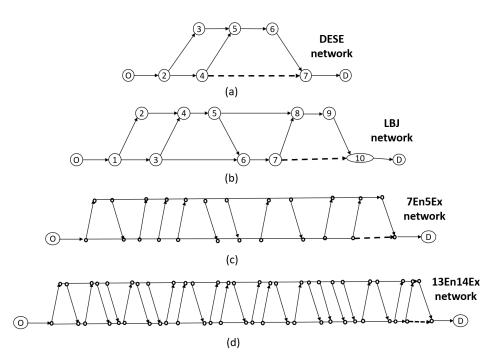
Figure 3.4: Four test networks: (a) double entrance single exit (DESE) network; (b) LBJ TEXpress network for toll segment 2; (c) a network with seven entrances and five exits (7En5Ex); and (d) a network with thirteen entrances and fourteen exits (13En14Ex). The dashed link indicates the location of downstream bottleneck.
