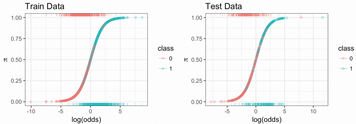
Figure 3.9: Logistic regression curves on train and test data. Sigmoid logistic regression probabilities versus predictions (i.e. log odds) on the train and test data, where class 0 (false) and 1 (true) strands are colored as red and green respectively.
