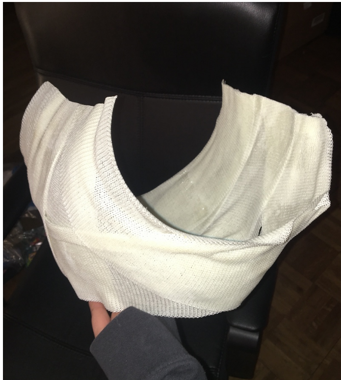
Figure 2.4: Front view (top) and isometric view (bottom) of cast after removing top flaps to get rid of undercuts for suitability for 3D scanning.
