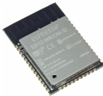
Figure 12: Espressif ESP32 SoC
