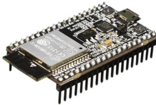
Figure 17: ESP32-DevKitC Breakout Board
