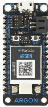
Figure 11: Particle Argon Development Board [19]
