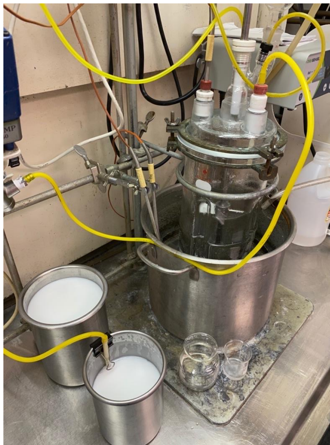
Figure 9. Monomer pre-emulsion, redox co-feed, and redox charge ready for synthesis. Initiator charge (front beakers) is added to the reactor, at which point monomer and initiator co-feeds are initiated. This particular setup is for a two-stage polymer, where the second larger emulsion will be fed following the completion of the first.
