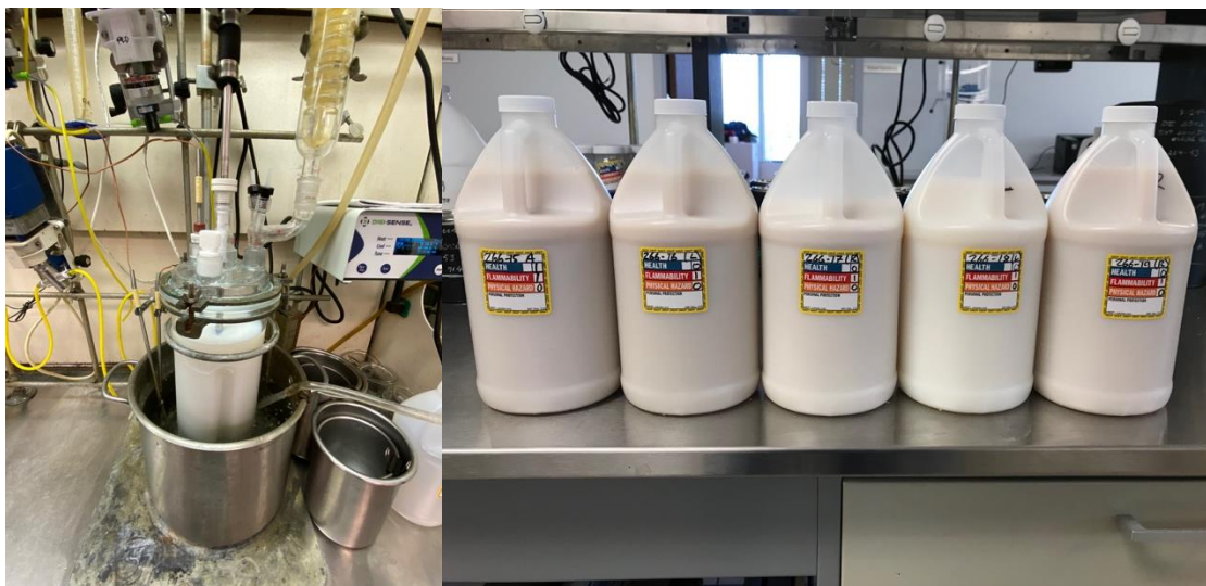
Figure 10. A finished emulsion reaction with polymer still in the reactor. At this point the product is filtered through a 100-micron filter into the jugs (left). A series of completed polymer resins (0.5 gallons) awaiting testing (right).
