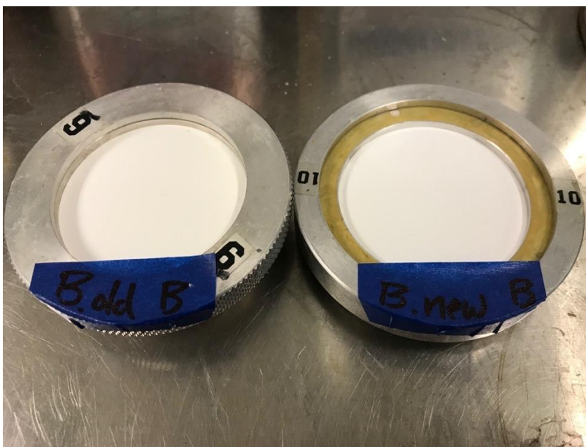
Figure 13. Films are cut out and placed in the BYK permeability cups. Note that these cups have slightly different designs but perform identically.
