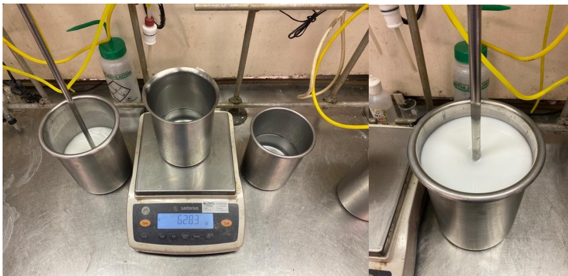
Figure 8. Monomer pre-emulsion building process (left). Monomer pre-emulsion complete and ready for reactor feed (right).
