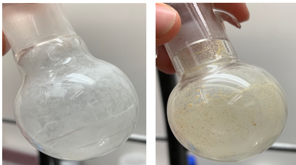
Figure 47: Inclusion complexes \beta CD-C12:AdSSPEG (left), and \beta CD-C14:AdSSPEGOMe (right) form thin films in round bottom flasks that are suitable for rehydration to form vesicles
