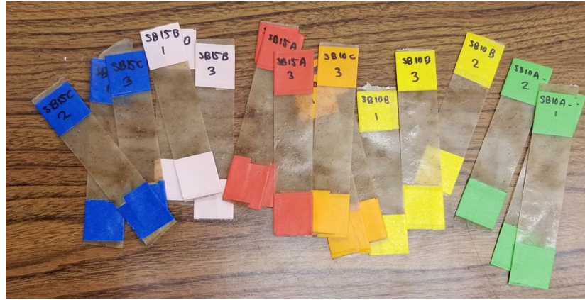
Figure 3.4: Peach flour -high-density polyethylene biocomposite samples for tensile testing
