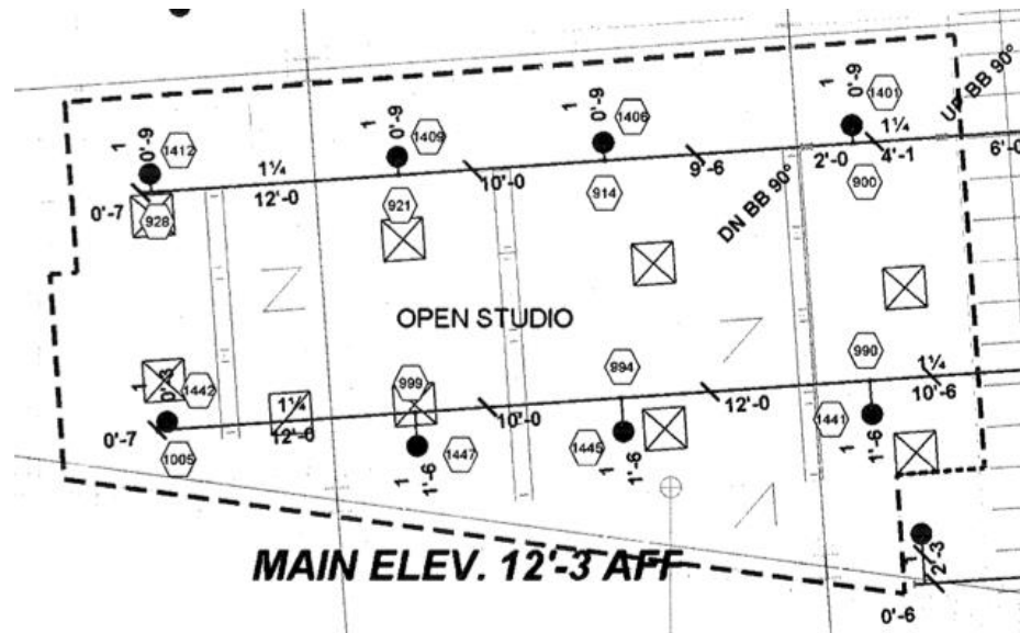
Figure 37. Hydraulically remote area on the first floor.
