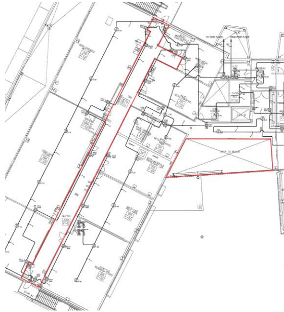
Figure 16. The unprotected area by smoke detectors
