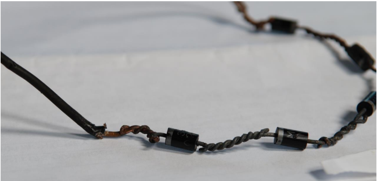
Figure 8: Negative end of chain from bath 1. This chain had been sanded at only the most positive and negative connections between the diodes and lead wires.
