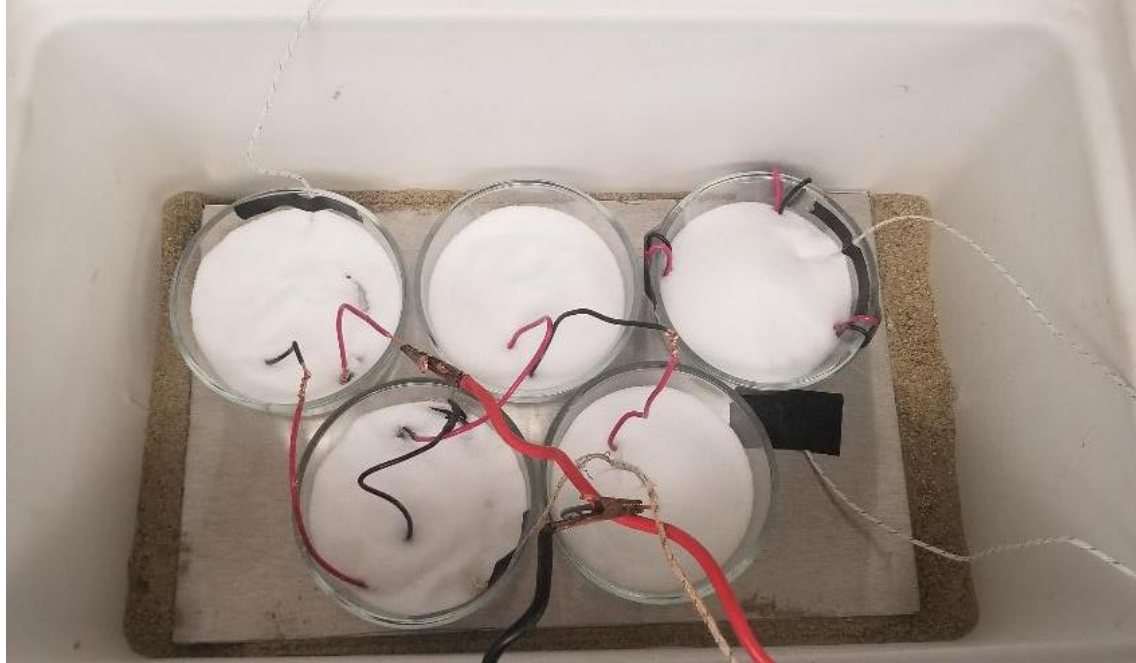
Figure 7. The cooler consisting of all baths filled with erythritol.
