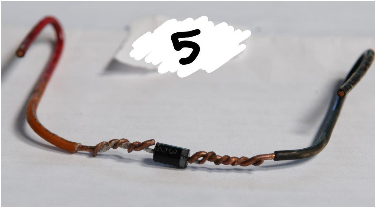
Figure 20: Diode with sanded leads from bath 5.
