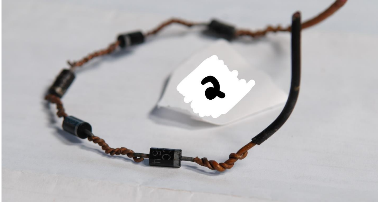
Figure 11. Negative end of chain from bath 2. This chain had all connections sanded to remove tin.
