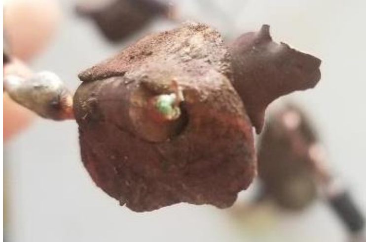
Figure 1. Corroded diode lead of a cooker constructed by twisting all connections. Surrounding the diode is erythritol and JB weld. During construction, diode bodies were glued to the pot using JB weld, but leads were left uncoated.
