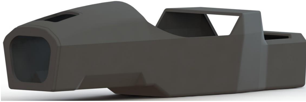
Figure 41. Refined preliminary geometry. Note the lower control arm boss added to the lower front of the cockpit and the flat shock “shelf” at the rear.
