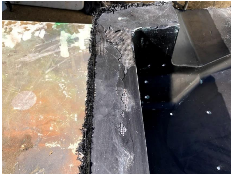
Figure 140. Surface coat cracking along the rearmost flange on the rear molds.
