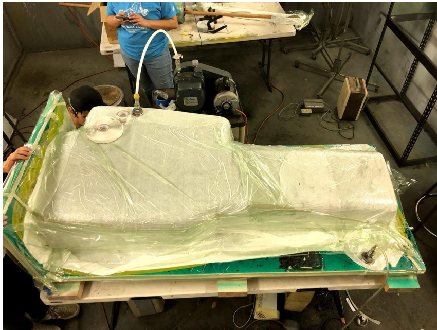
Figure 136. FR mold inner skin being debulked.
