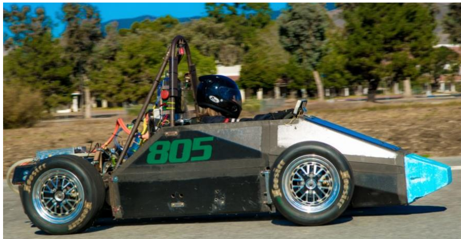
Figure 11. 2015 Frame Engineering Associates cut-and-fold chassis.
