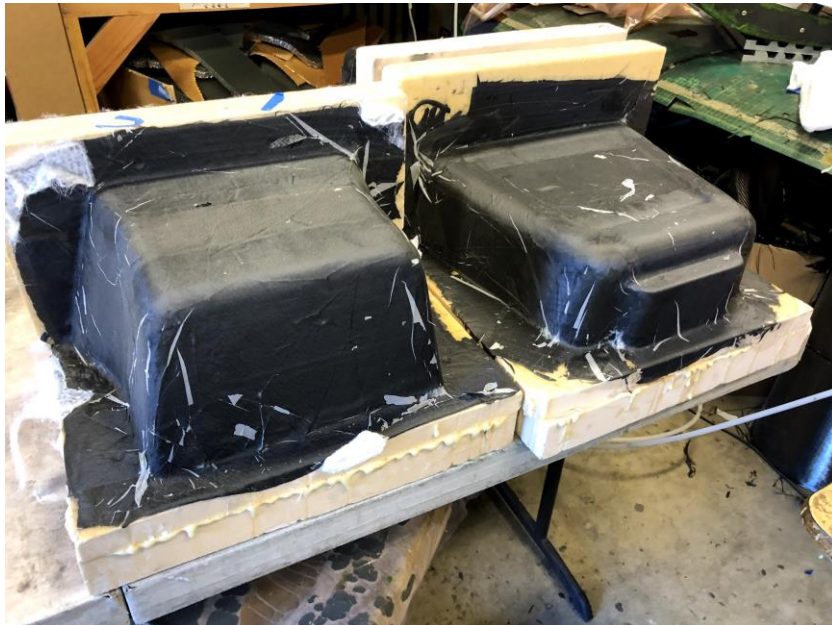
Figure 108. Cured carbon molds not yet released from the plug.
