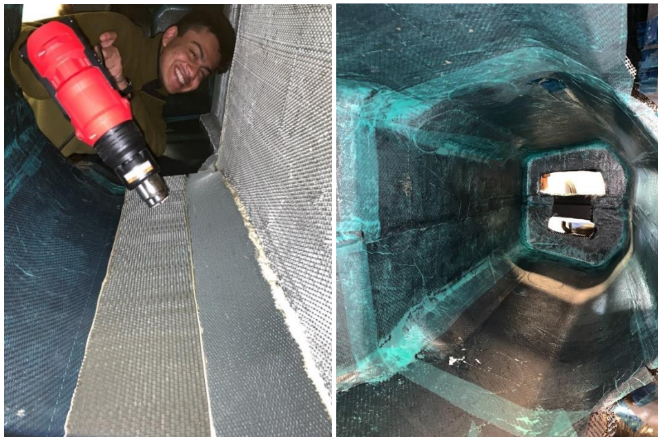
Figure 165. Heating the film adhesive (left) after contaminating the film adhesive from debulking (right).
