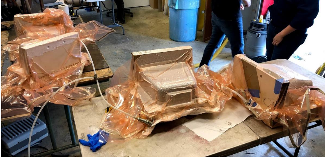
Figure 107. Each of the baby mold quarters curing under vacuum.
