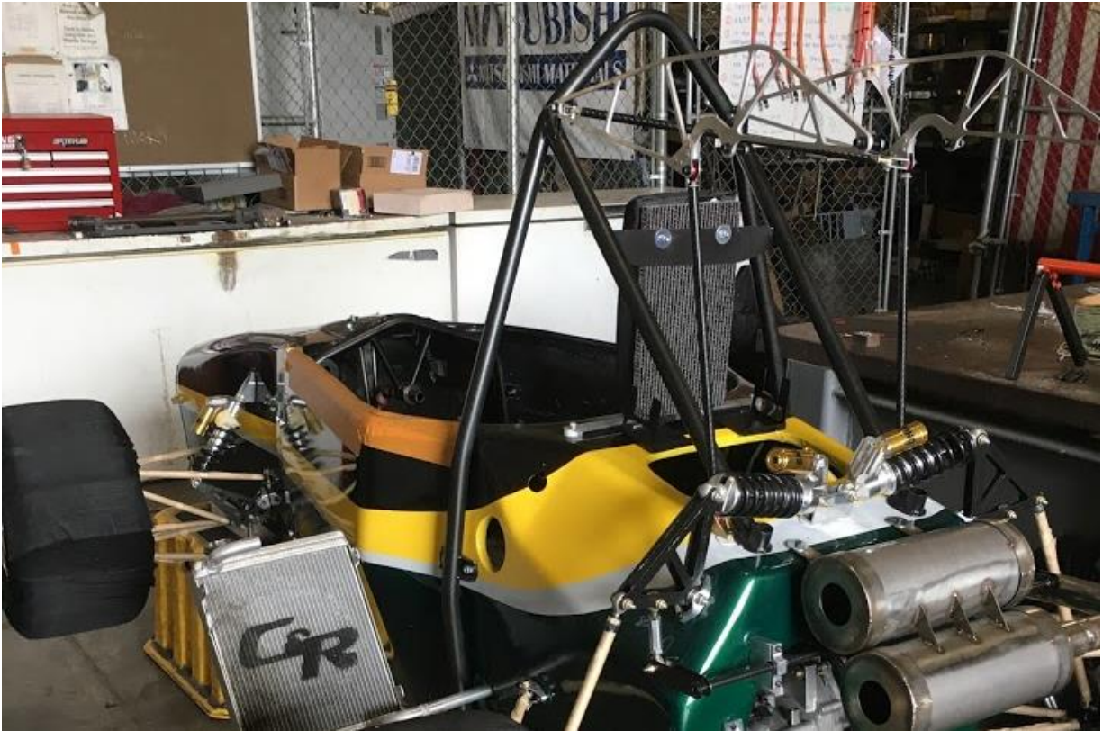
Figure 73. CPFSAE 2019 main hoop bracing configuration.
