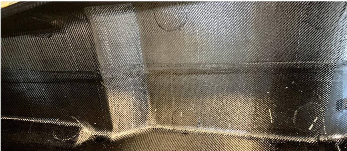
Figure 175. Seam down the centerline of the monocoque floor.
