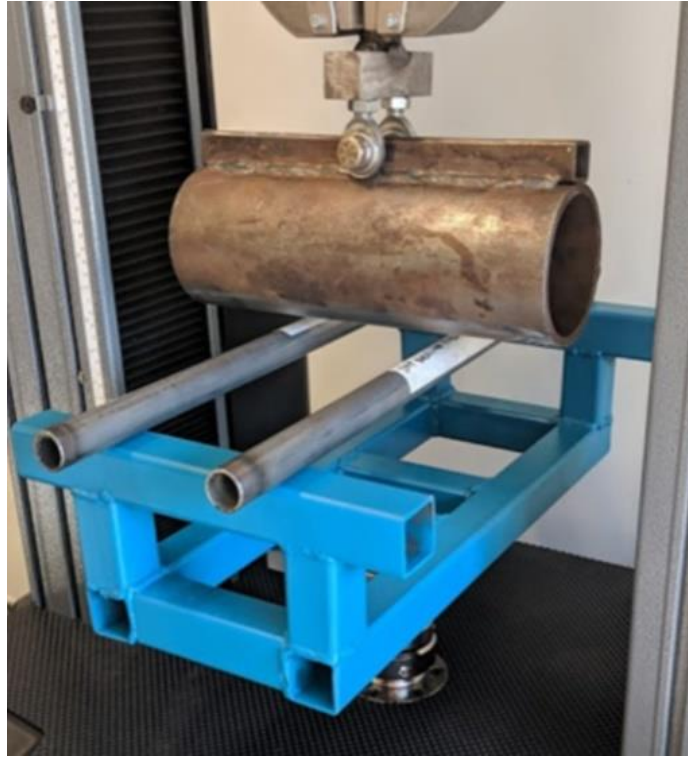
Figure 65. Steel tube baseline 3-point bend test setup.
