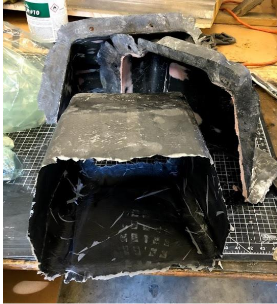
Figure 113. Successful male part pulled from two baby mold halves.
