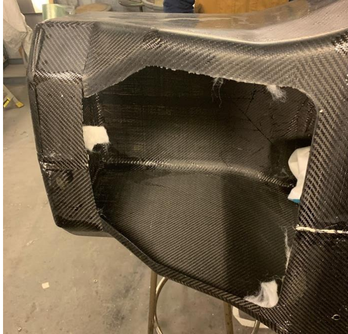
Figure 155. Released single ply skin at the rear mold.
