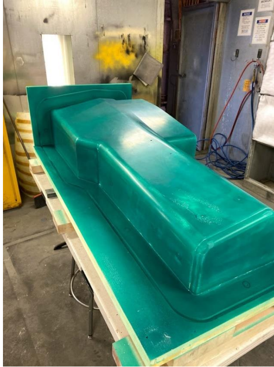
Figure 131. Sealed and sanded PVC Lacquer layer on the FR plug.
