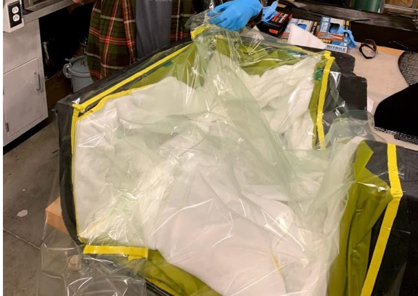
Figure 158. Localized vacuum bag on the inner surface.
