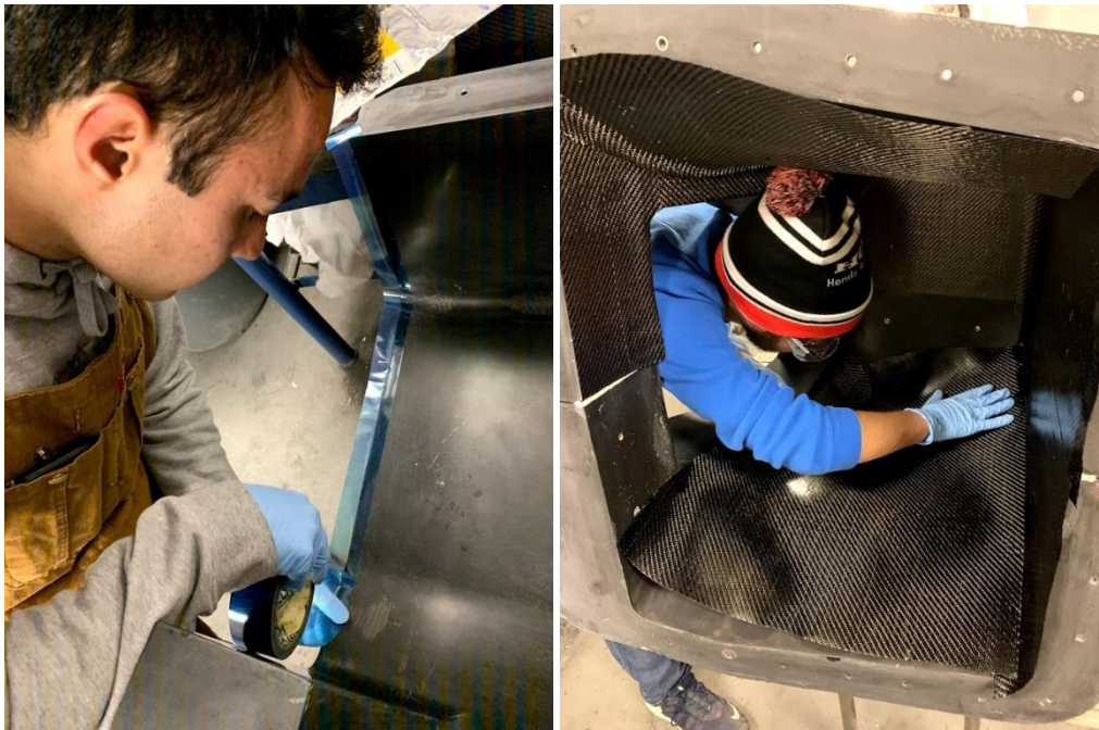
Figure 150. Flash tape as a bridge between mating mold pieces (left), verifying function of the access holes during a layup (right).
