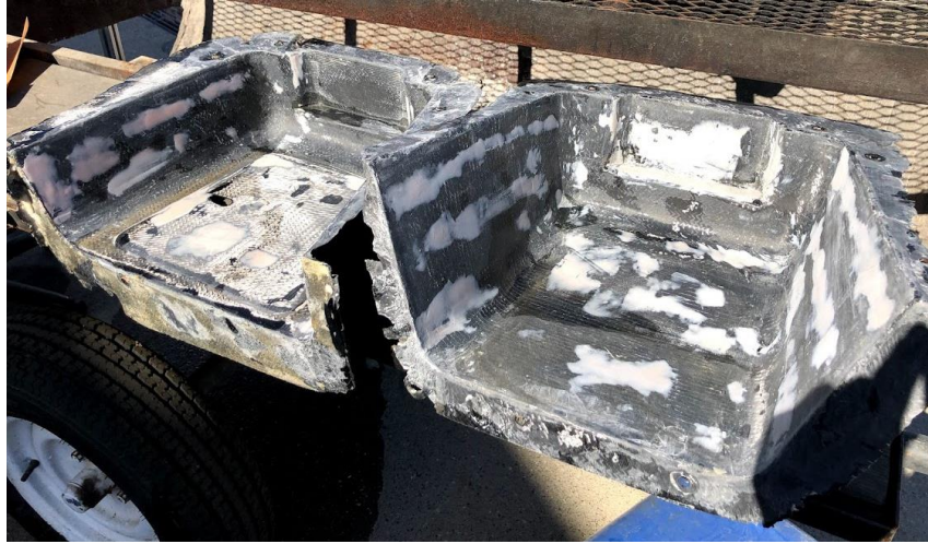
Figure 111. Sanded and cleaned female mold halves of the baby mold.
