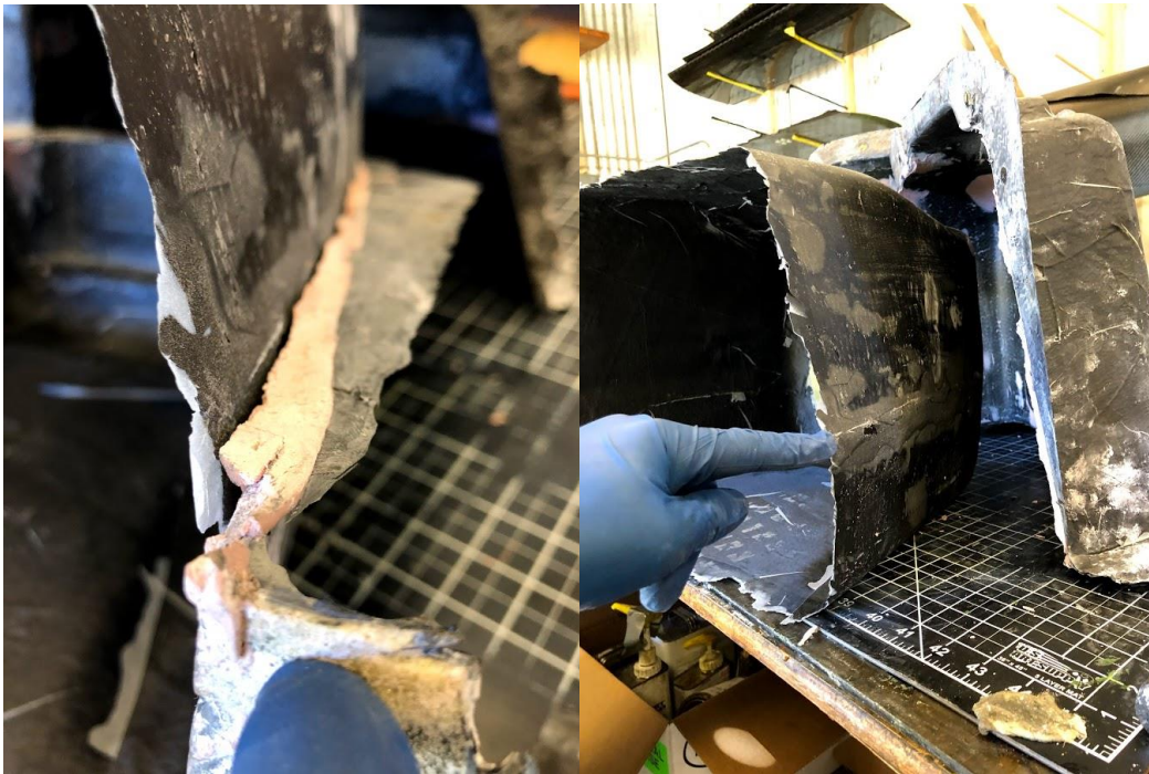
Figure 114. Bondo seam had to be broken using a chisel to disassemble mold halves (right). No cusp exists on the final part (left).
