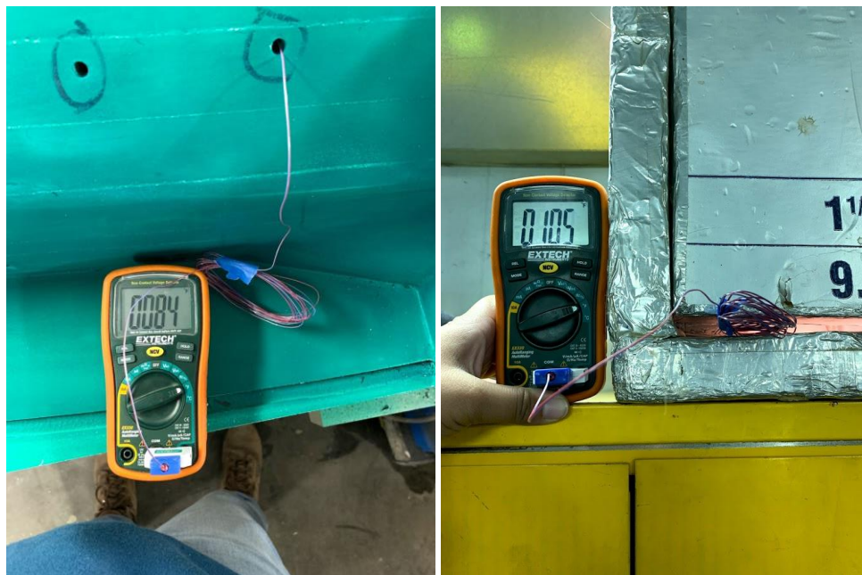
Figure 133. Room temperature determined by measuring thermocouples inserted within the foam (left), warmer box temperature determined by measuring thermocouples inserted into the box (right).
