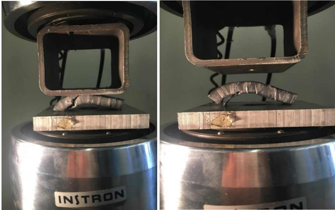
Figure 61. Images of single-stage cured sample pieces after destructive testing.
