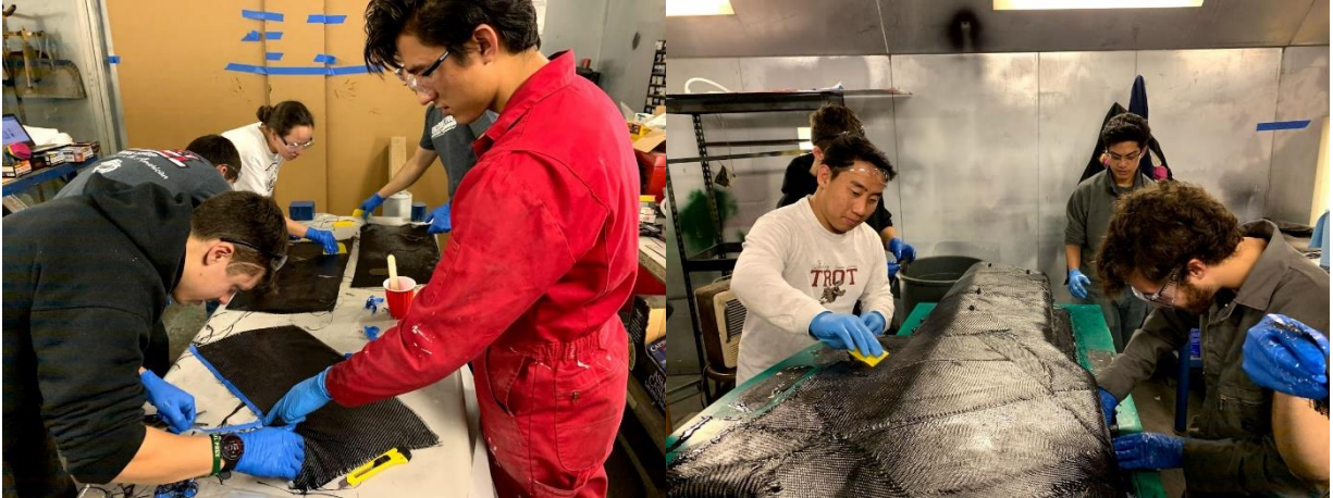
Figure 135. Wetting out carbon and removing masking tape (left), applying wet carbon and squeegeeing out air (right).
