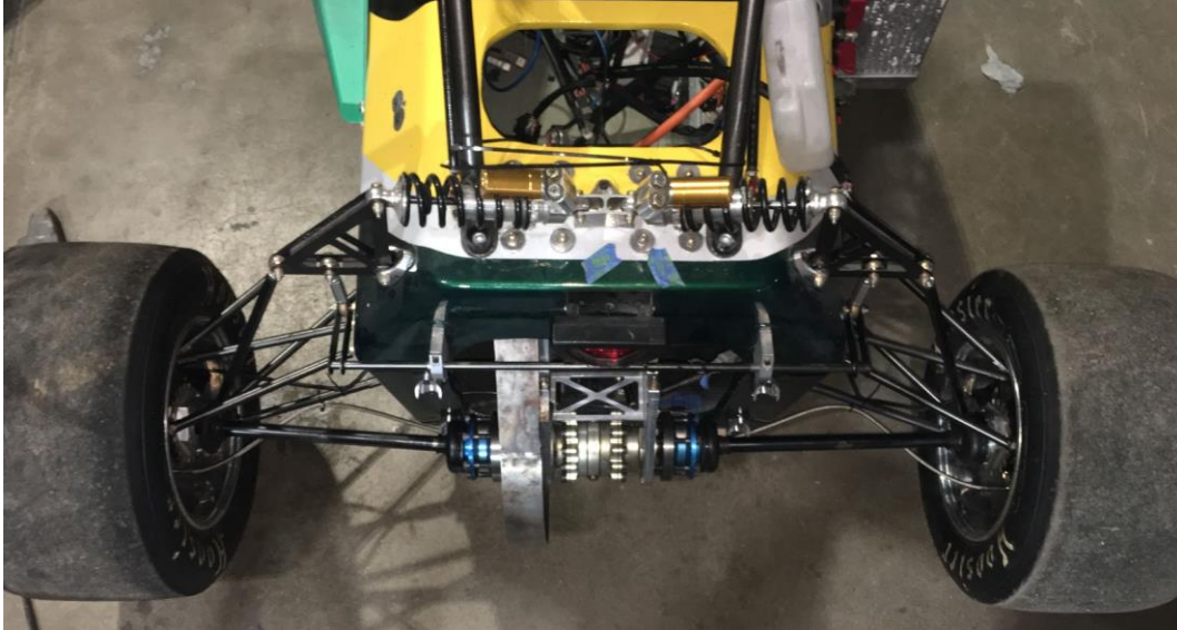
Figure 33. 2019 suspension geometry with in-plane rockers and double shear mounts.
