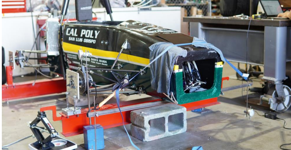
Figure 185. Chassis torsional stiffness test rig. Notice the scissor jack applying load to the FR jig, while a dial indicator measures the displacement of the FL jig.
