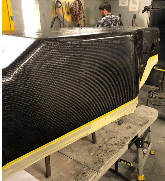
Figure 186. The combustion car chassis being painted before campus closure.
