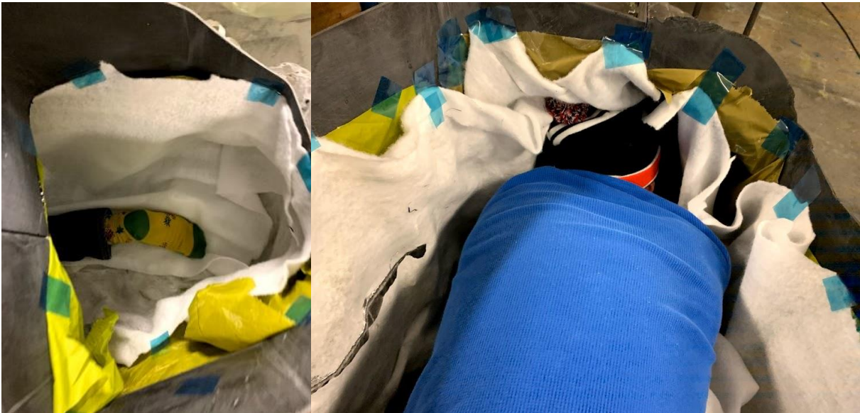
Figure 152. Attaching breather and release ply.
