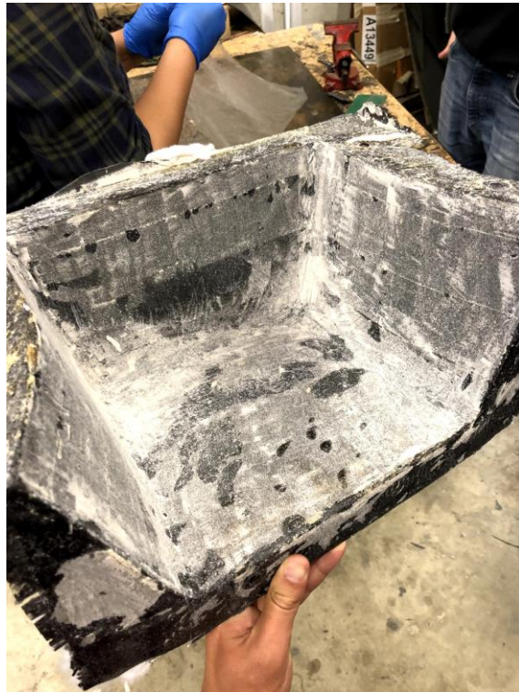
Figure 110. The inside of the carbon fiber baby mold quarter.
