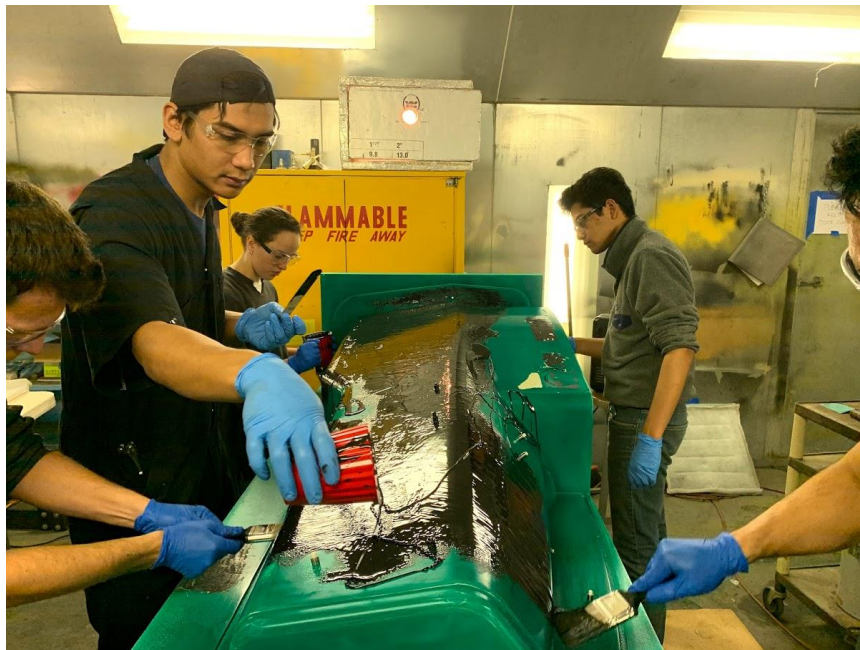
Figure 134. Application of the surface coat in a thick layer.
