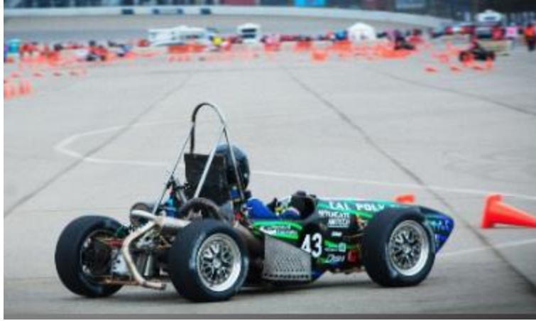
Figure 10. 2013 Formula Chassis Works partial monocoque chassis at competition.
