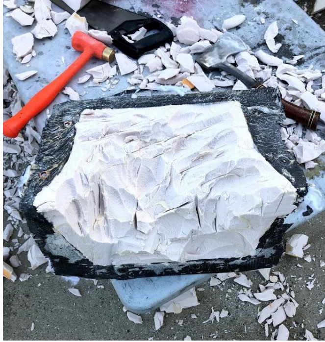
Figure 109. “Releasing” the carbon mold from the plug.
