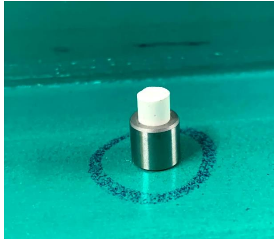
Figure 119. Resin pin and steel bushing in male plug before layup of female mold.
