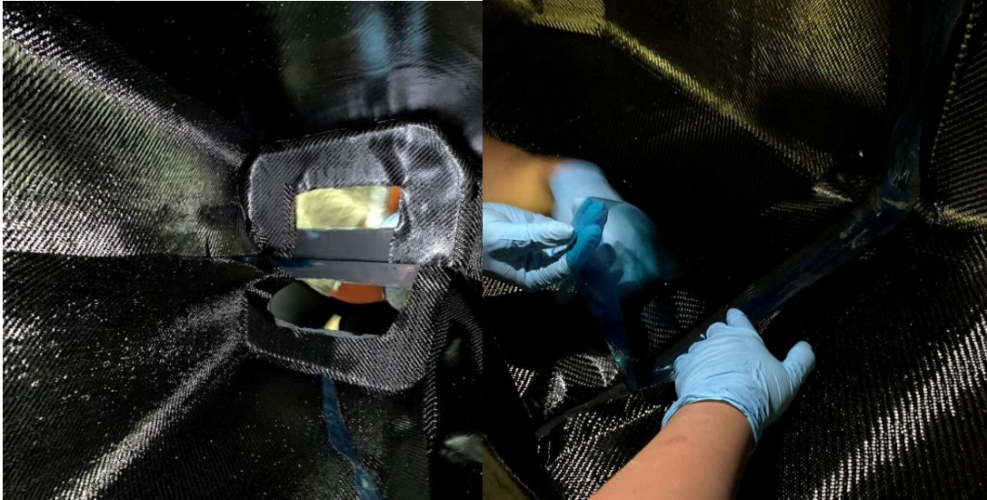
Figure 151. Unmated seam between the front quarters (left) and attempt to apply flash tape under overlapping plies.
