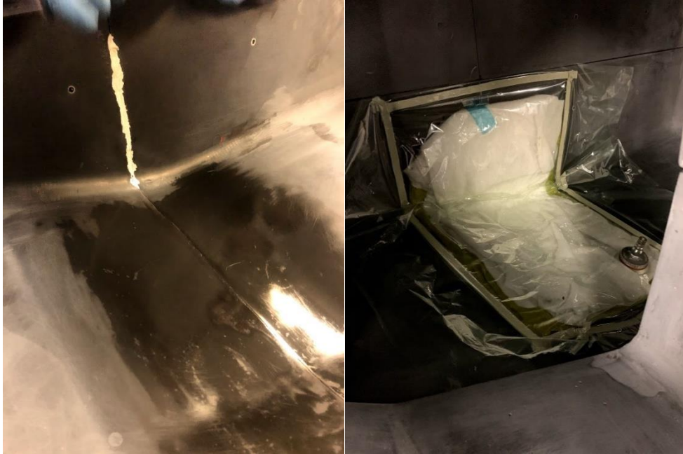
Figure 149. Plasticine filled and unfilled mating lines (left) lie underneath the test layup (right).
