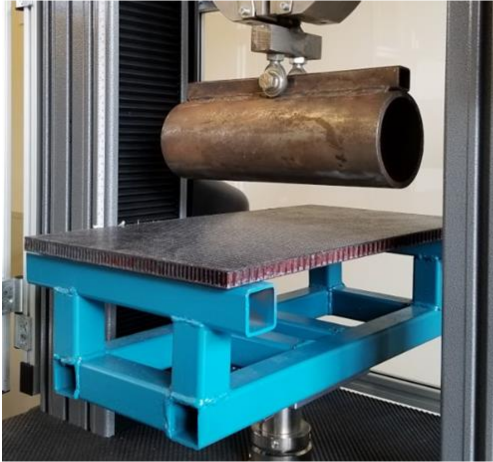
Figure 9. 3-point bend test setup for SES.
