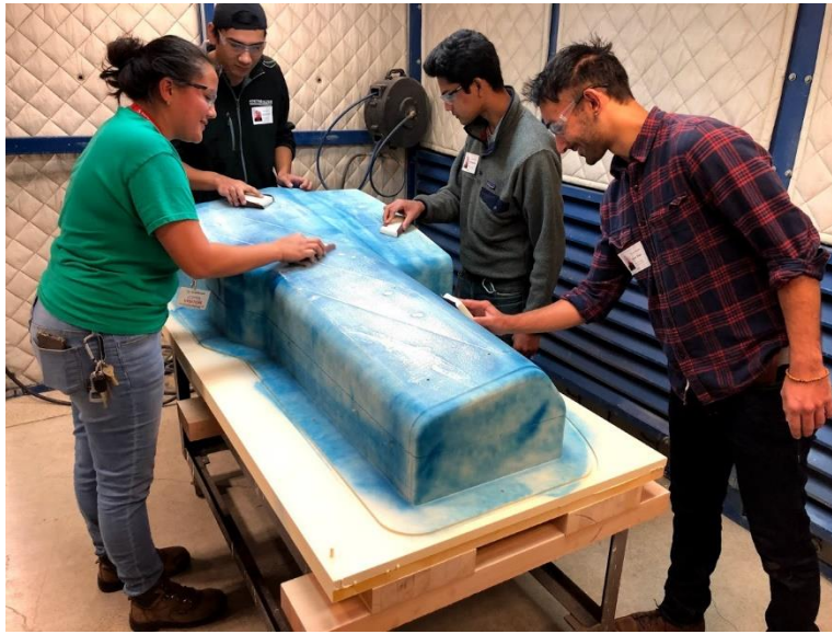
Figure 130. MCD team and CPFSAE team volunteer beginning to sand the FR foam plug.
