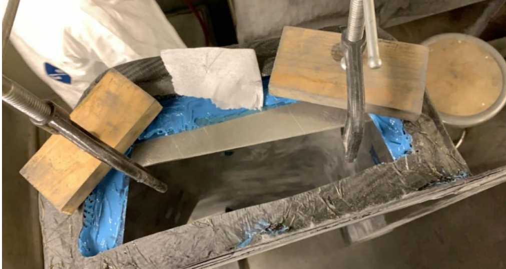
Figure 146. Front bulkhead fill in procedure. Loctite 9396 was first applied and cured, then a mix of Loctite 9396 and chopped fiber was added for extra structure.
