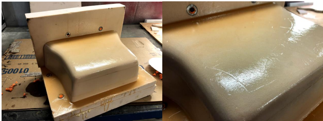
Figure 106. The resin sealed foam plug with drill bushings (left). The orange bits are earplugs used to keep resin out of the drill bushing holes. The rough, undesirable resin surface is shown on the right.
