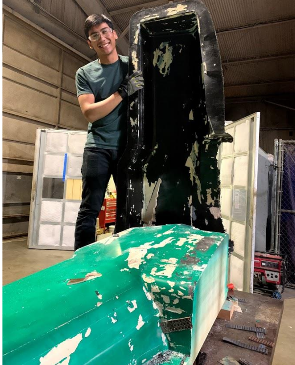
Figure 139. Removal of the FR mold from the plug. Notice the severely damaged plug and adhered foam on the surface coat.
