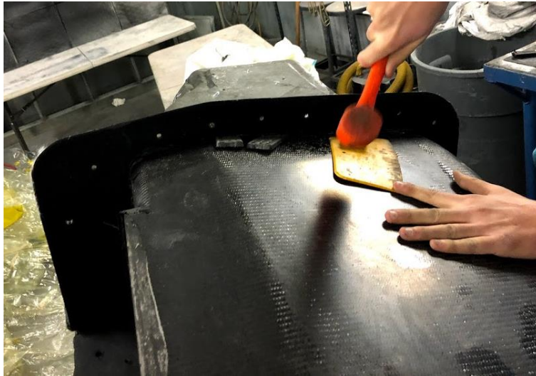
Figure 169. Wedging under the RL (left) and released surface (right).
