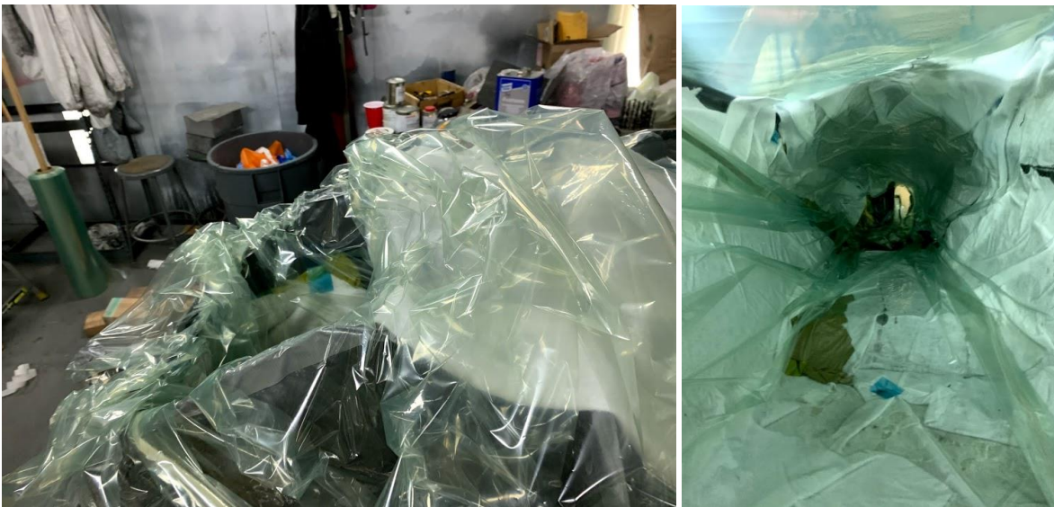
Figure 154. Donut bag through powertrain bay (left) and vacuumed bag (right).
