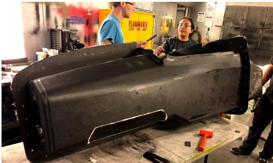
Figure 168. Removal of the FL mold piece. The plasticine used the seal the corner around the FLCA surface insert baked onto the chassis structure.
