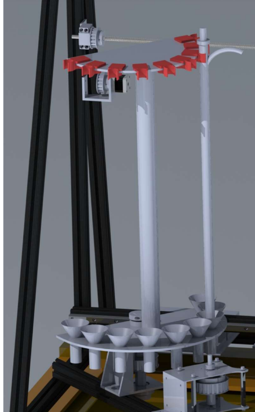
Figure 10. CAD Model of Concept Design Tool Changer Mounted to STYX Frame
