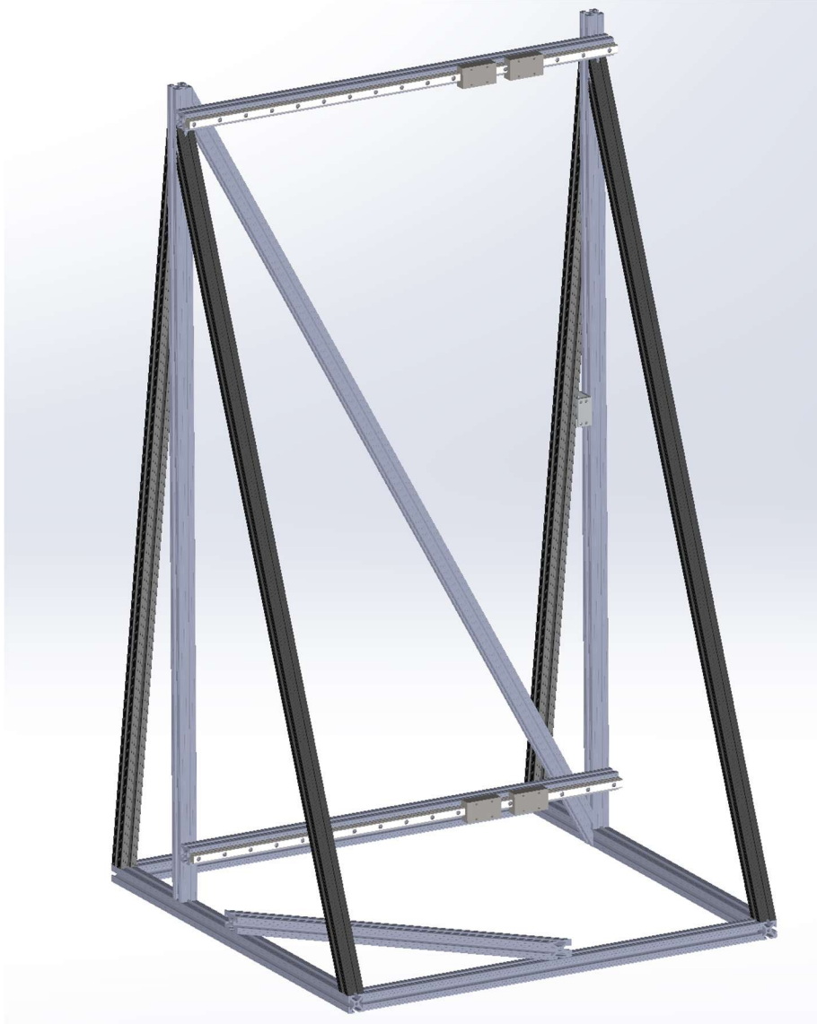
Figure 17. Frame concept design A frame X-rail.
