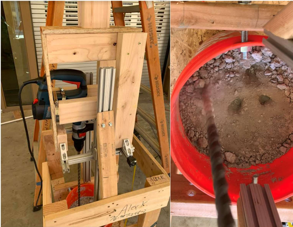
Figure 7. Test Stand for Drilling Process
