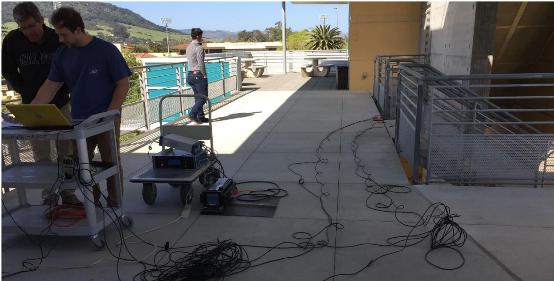
Figure 1. Forced Vibration Testing Equipment and Setup
