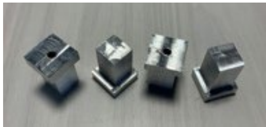
Figure 8. Completed End Caps
