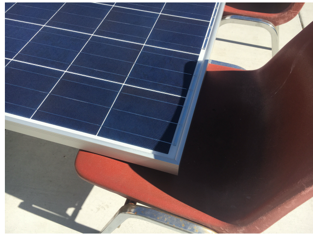
Figure 8.6. Shading from test 5 (Panels flat on ground)
