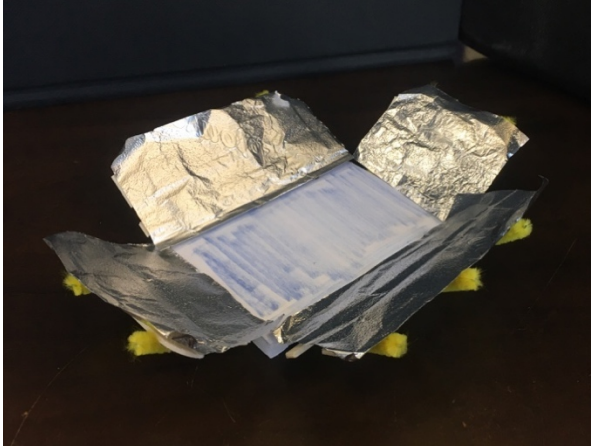
Figure 4.5. Mirror design for extra sunlight on solar panels.
