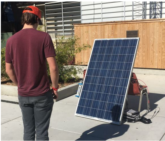
Figure 8.5. Shading ( \approx 9 \text{ in}^2 ) used in test 2 (Panel normal to the sun).
