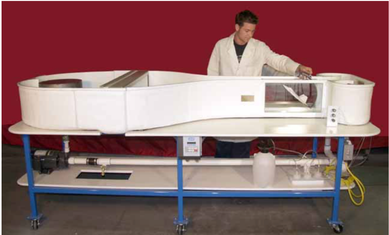
Figure 2.12. Rolling Hills Research Corporation Model 0710 University Desktop Water Channel used for propeller design verification.
