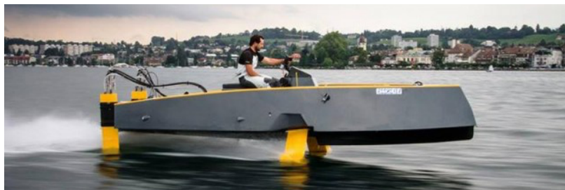
Figure 2.3 Motorboat powered by a hydrofoil system.
