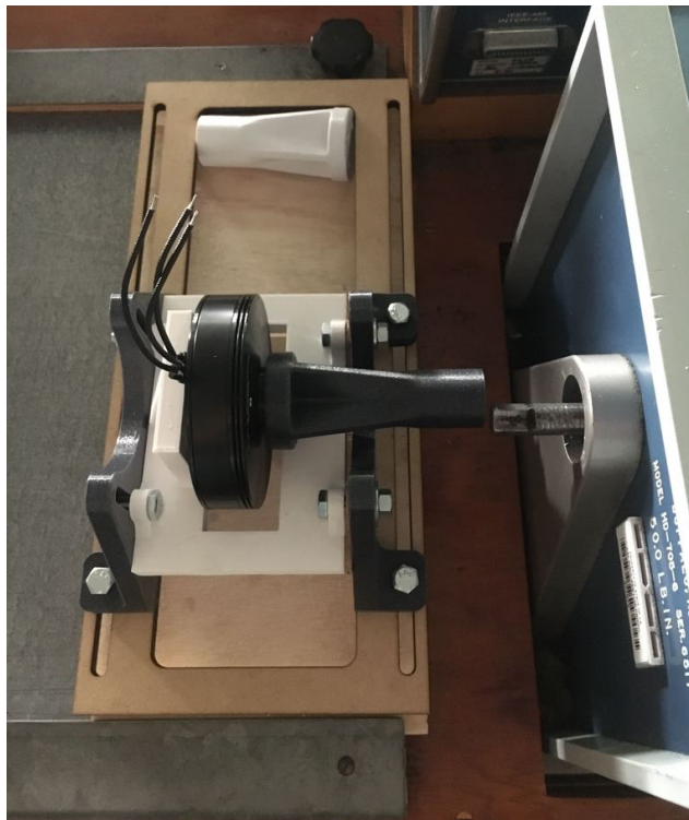
Figure 8.2. Motor test jig setup with dynamometer.
