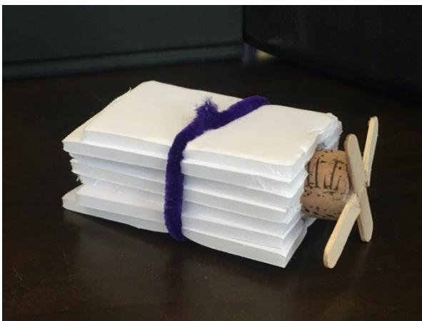
Figure 4.3. Prop inside hull pontoons.
