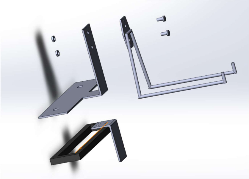
Figure 30. Exploded View of Wheel Storage Device.
