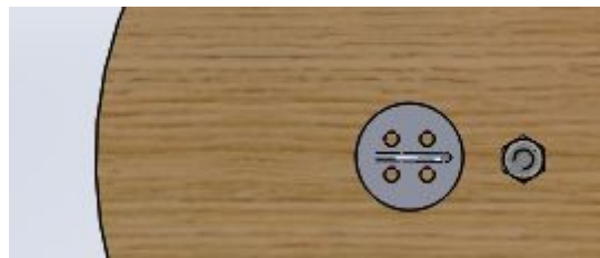
Figure 2.3: Speedbag Swivel Mount Bolted to Wooden Plate
