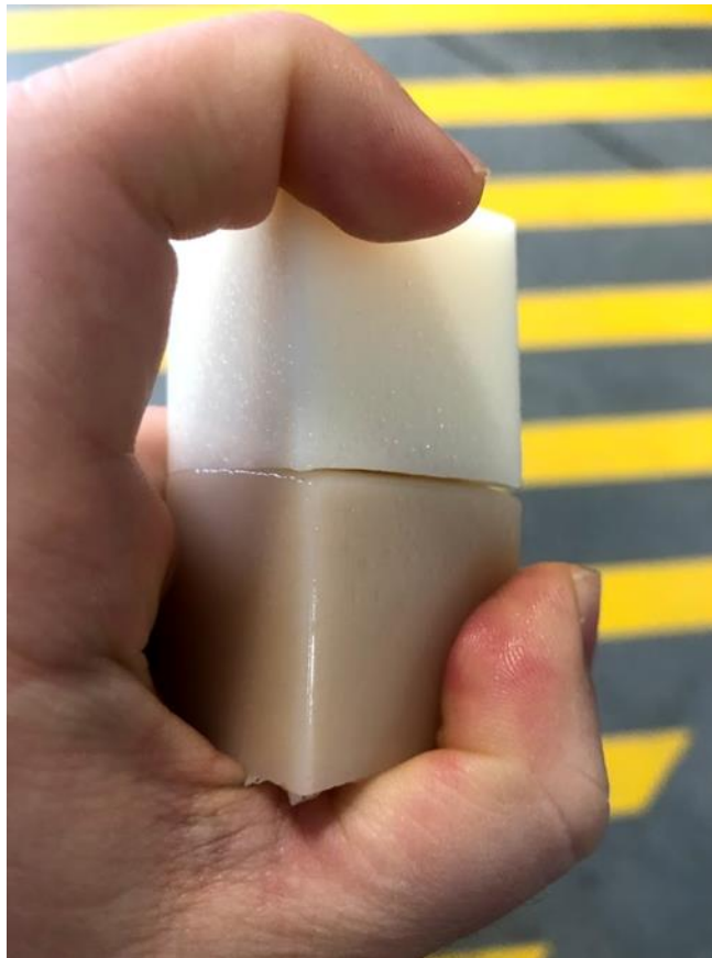
FIGURE 7.1 INCOMPLETE ADHESION WHEN BOTTOM LAYER CURED TOO LONG
