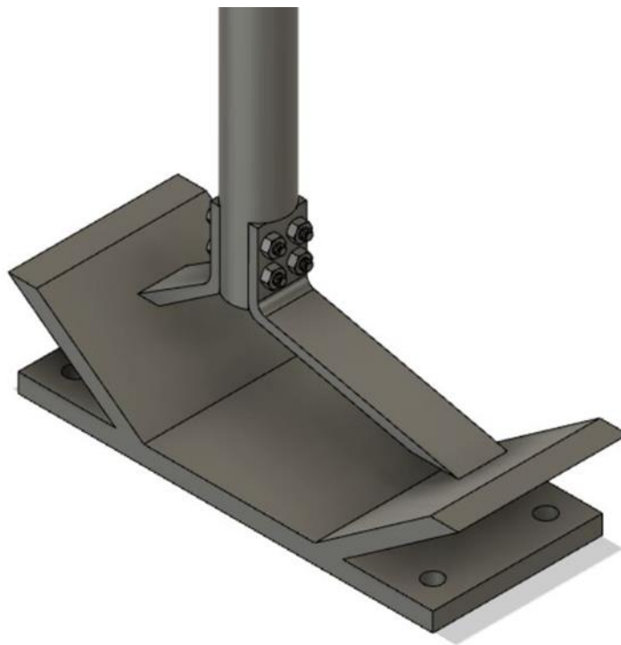
FIGURE 7.2 POSSIBLE FATIGUE TEST FIXTURE DESIGN, INCLUDING BASE PLATE
