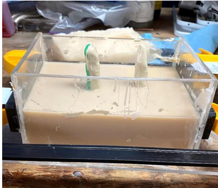
FIGURE 6.4 MOLD BOX CONTAINING TWO URETHANE LAYERS AND SPRUES
