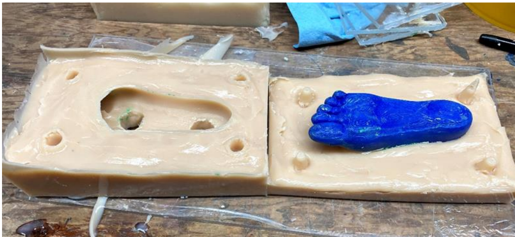
FIGURE 6.5 FINAL PRODUCT OF OUTER MOLD FOR FOOT SHELL
