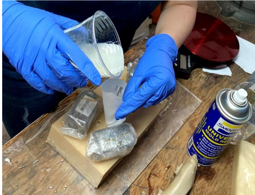
FIGURE 6.10 POURING THE PMC 770A INTO THE OUTER MOLD
