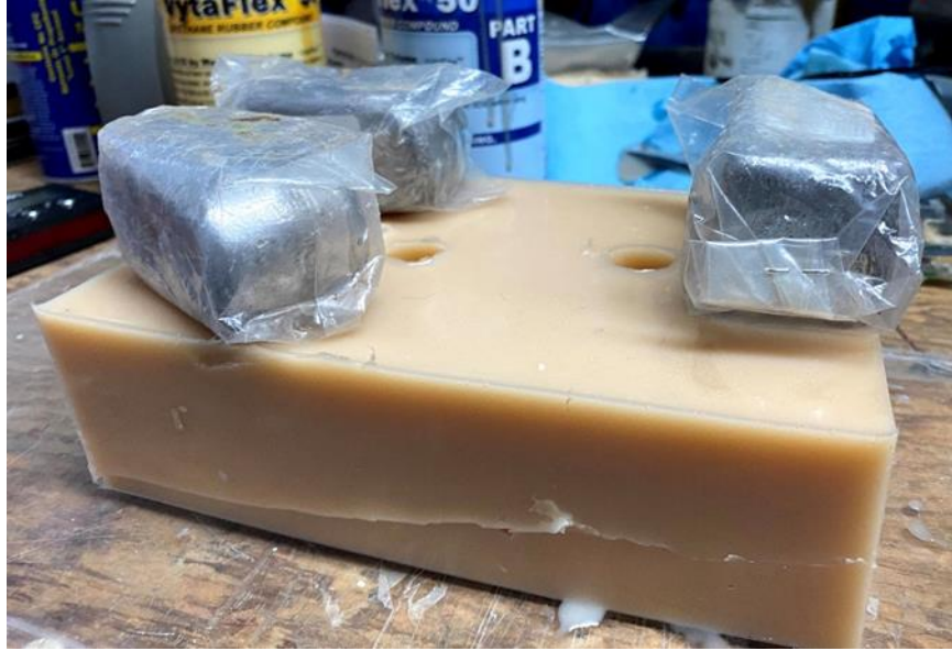
FIGURE 6.9 OUTER MOLD PUT TOGETHER WITH WEIGHTS ON TOP
