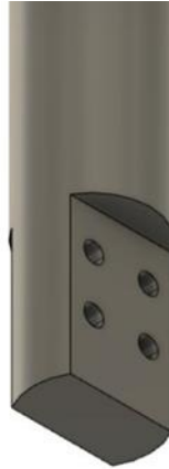
Figure 2. Shaft with the necessary \frac{1}{4} " drilled holes made in steps 2 and 3.
