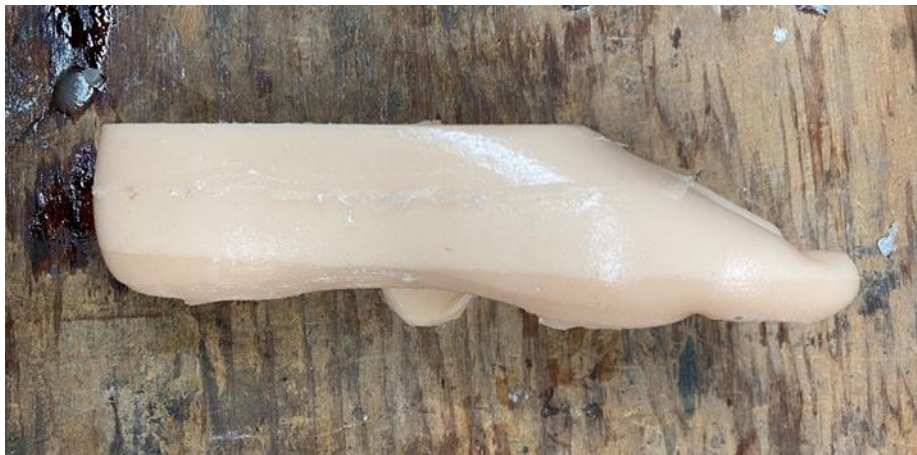
FIGURE 6.11 FINAL SCALE MODEL OF FOOT SHELL
