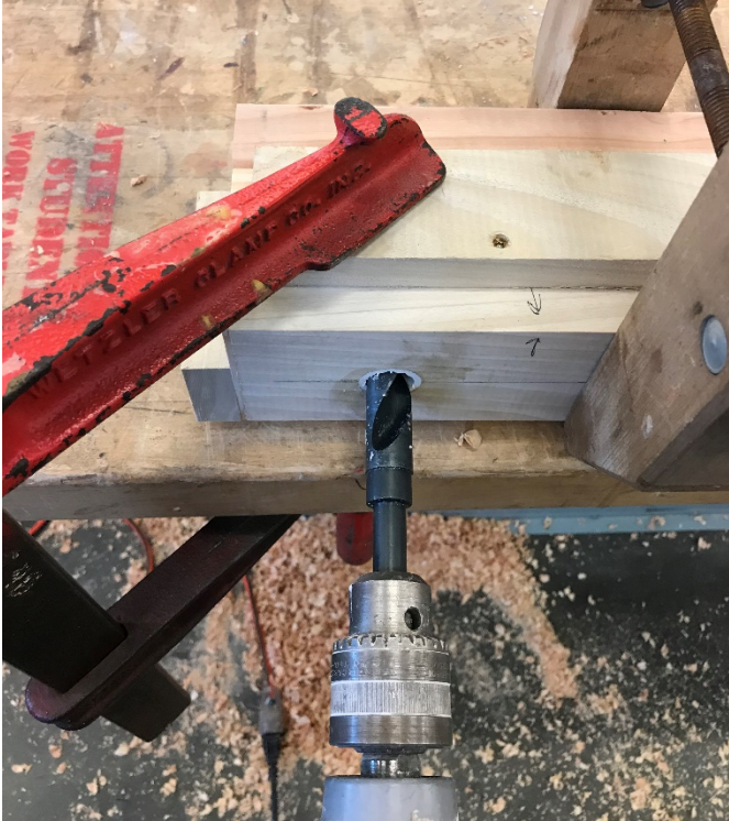
Figure 9: Drilling Holes in Boards Using the Jig as a Guide
