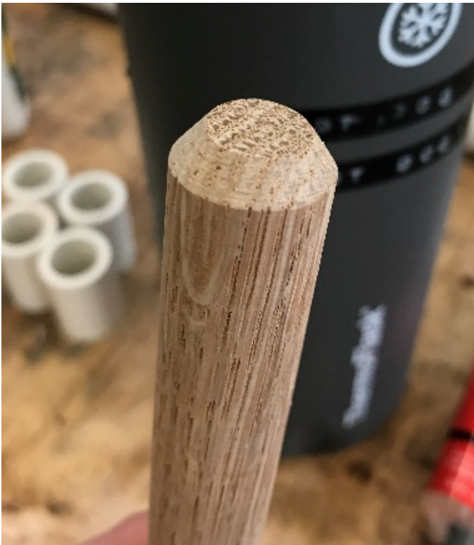
Figure 7: Chamfered End of Dowel
