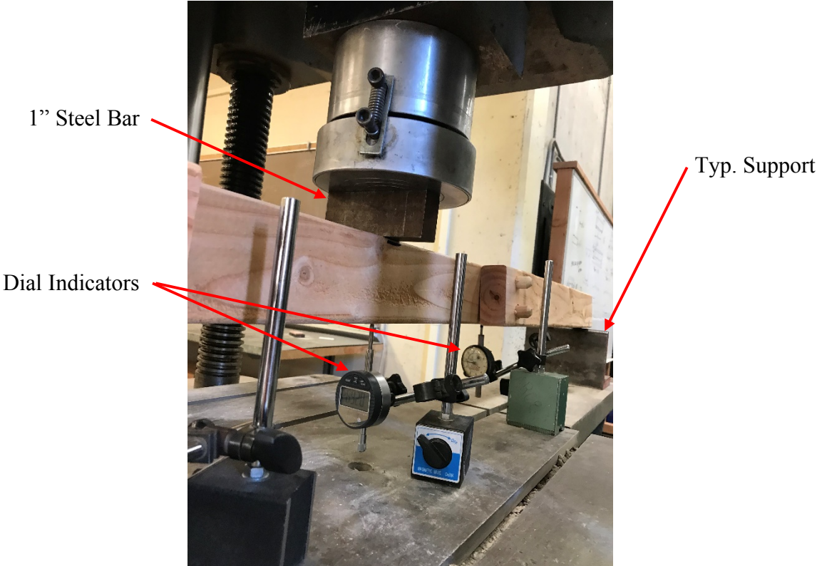
Figure 14: Baseline 2 Specimen Test Set-Up
