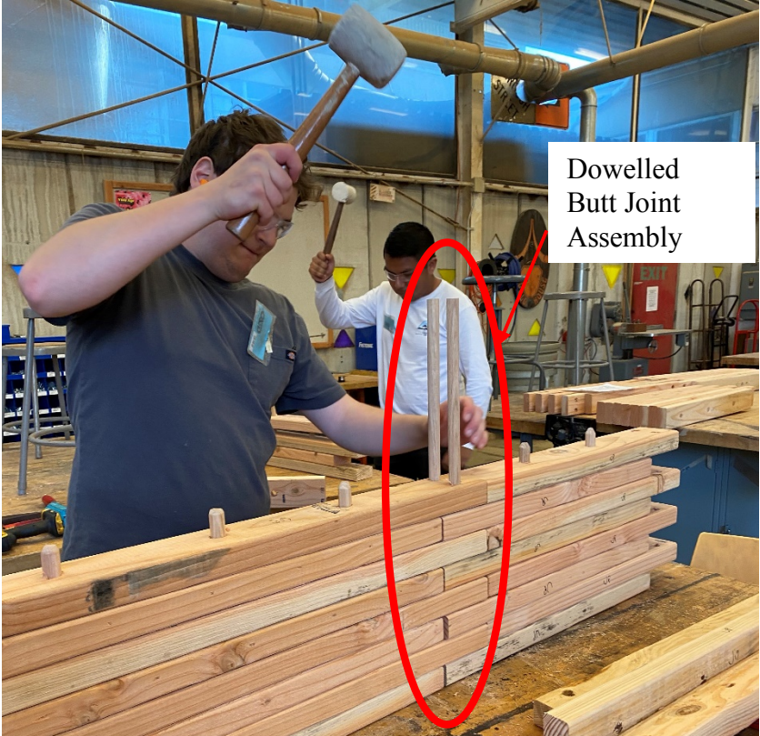
Figure 11: Joining DLT Panels by Inserting Butt Joint Dowels
