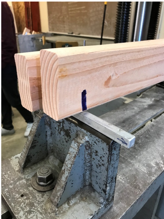
Figure 16: Example of a Shim Used for a Baseline 2 Specimen Test
