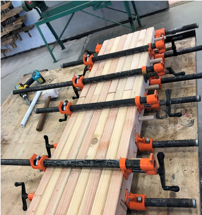
Figure 12: Clamping DLT Panel Overnight to Equalize Wood Moisture
