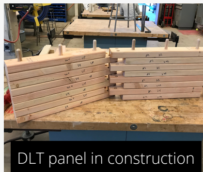
Reiley assmbling DLT panel
