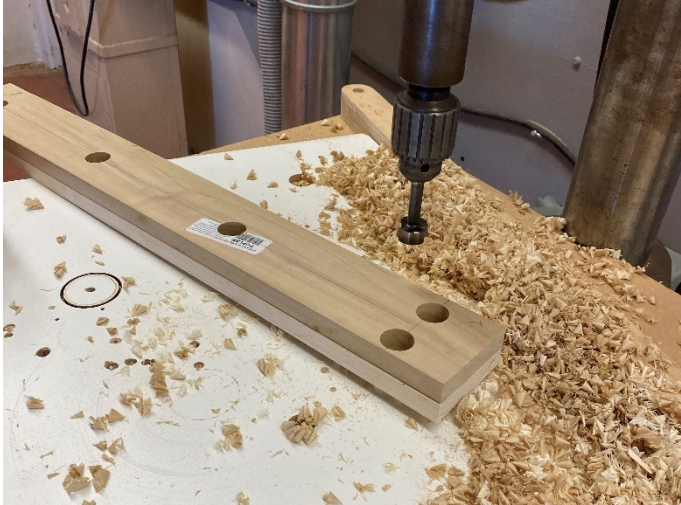
Figure 5: Drilling Holes to Accept PVC Pipe Bushing
