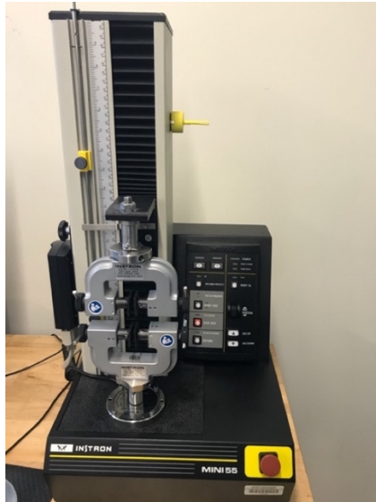
Figure 7 - Mini Instron 55 is used for smaller tensile specimens.
