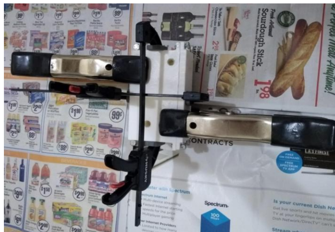
Figure 19. Set up of heel-side rubber mold before pouring liquid urethane
