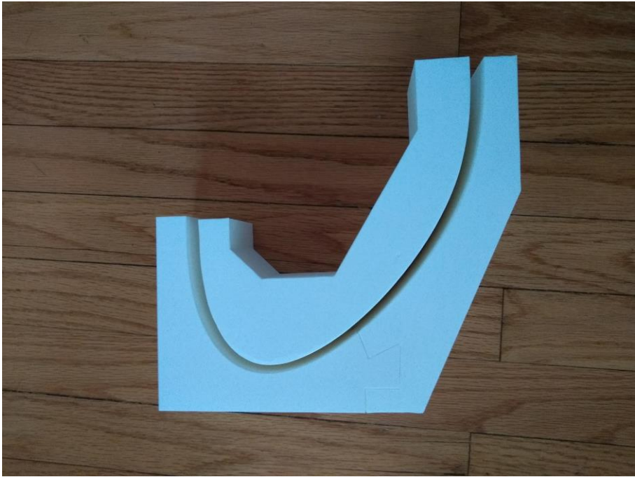
Figure 43. 3D printed pylon mold
