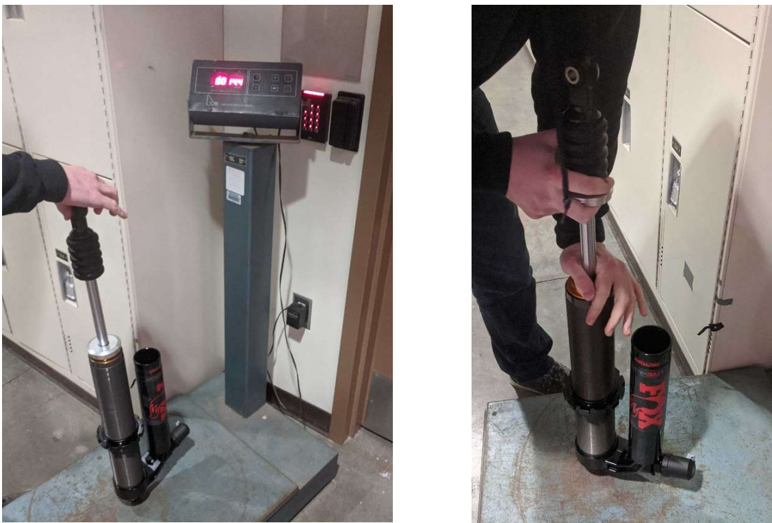
Figure 4-14. Shock weighing and preliminary O-ring compression quantification (Left and right images, respectively)
