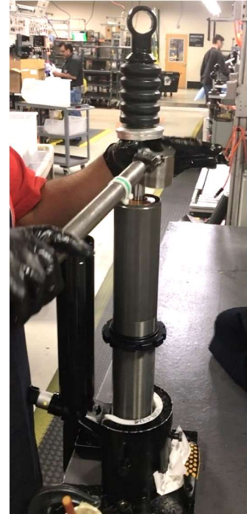
Figure 1-1. Manual rundown and torque process [1]
