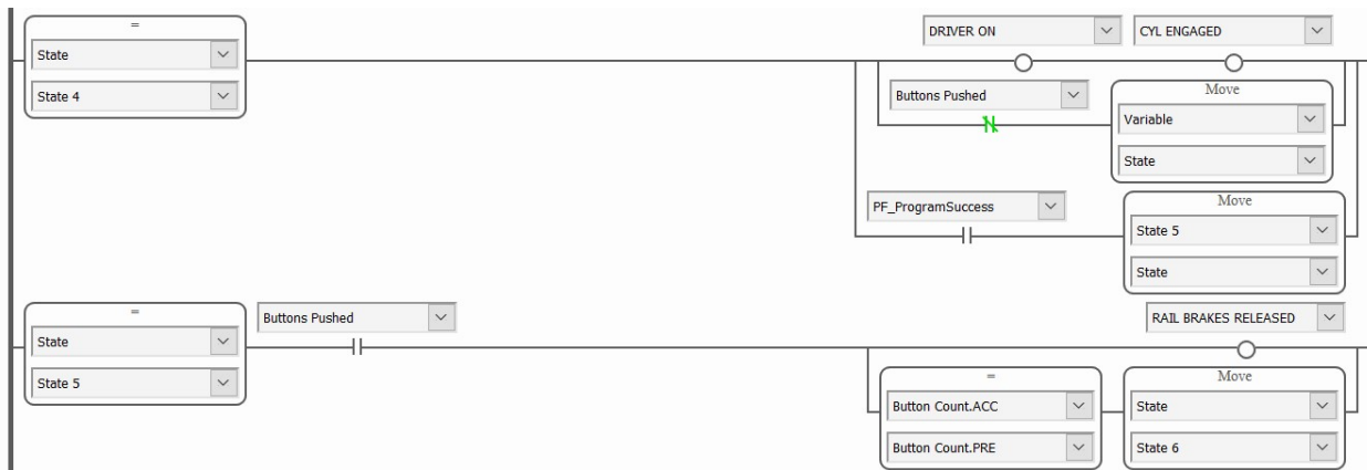
Figure 5-54. PLC Fiddle ladder diagram sample rungs
