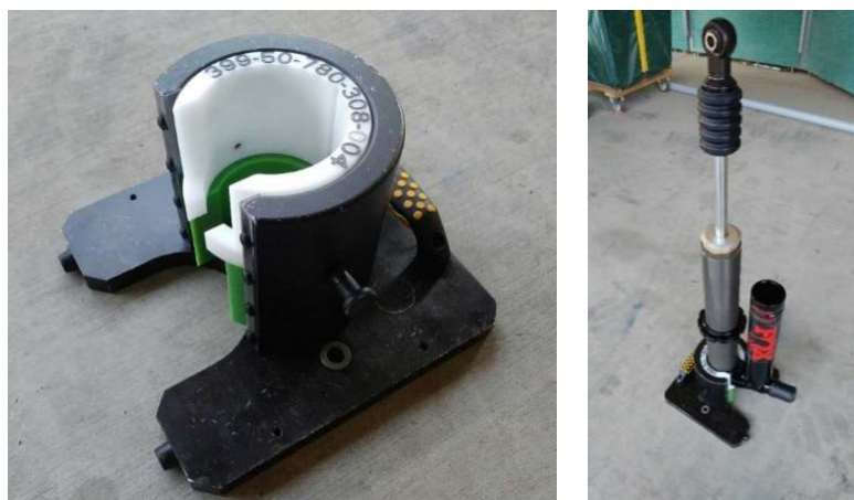
Figure 2-2. Body cap pallet assembly and pallet with shock loaded (Left and right images, respectively)
