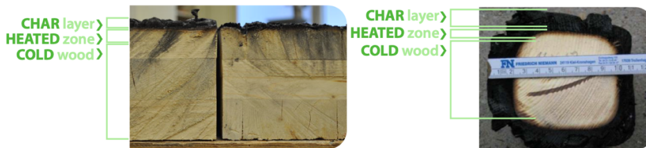
Figure 3: How Charring Protects Timber in a Fire Source: Fire Performance, reThinkWood
