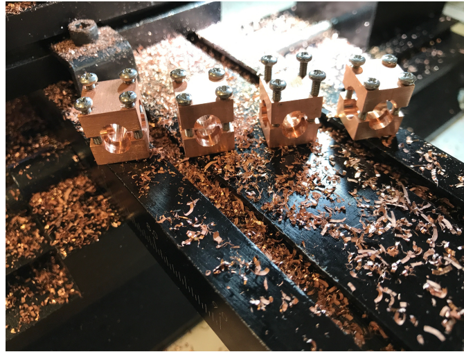
Figure 5.1: Transmission Line Cross Pieces
