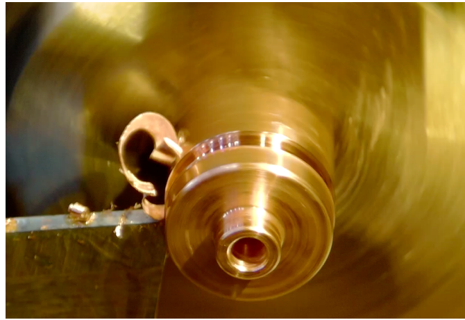
Figure 5.5: Turning a Shorting Plug
