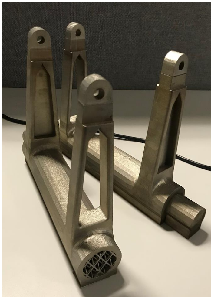
Figure 12a. Brackets Printed in 316L Stainless Steel
