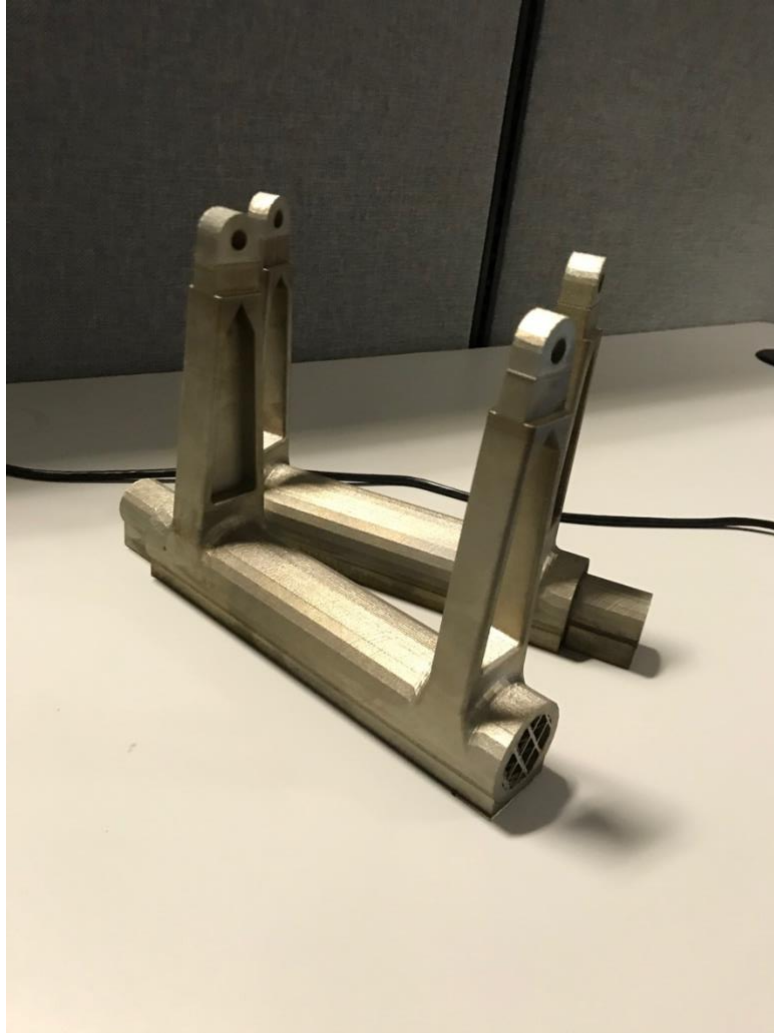
Figure 12b. Brackets Printed in 316L Stainless Steel
