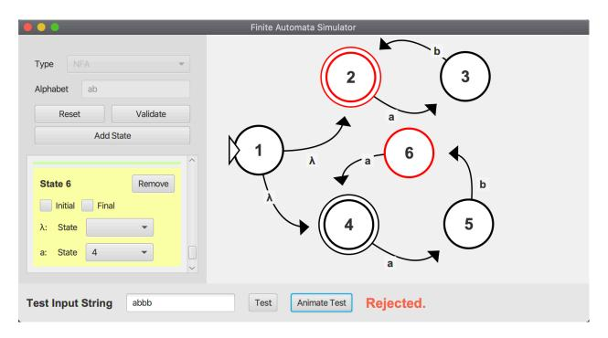
If the input string cannot be processed completely, i.e. there is an alphabet symbol that cannot be scanned/read from any of the states the NFA is in at the moment, the execution will stop and a result of "Rejected" will be displayed. The above example shows the NFA stopping execution at State 2 and State 6 on the second "b" symbol of the input string, leaving the "bb" postfix unable to be processed.
