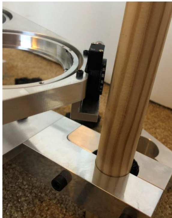
Figure 7.1. Clearance Achieved in Fit Test (3 mm)
