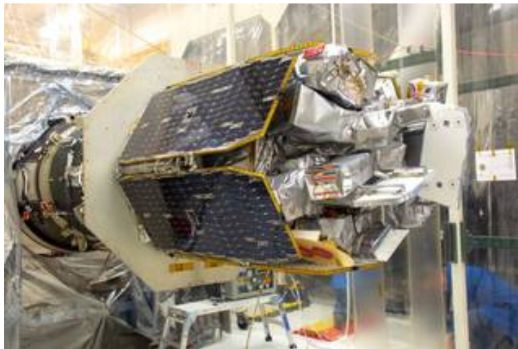
Figure 2.2: NASA ICON mounted to a Northrop Grumman Pegasus IV [13].
