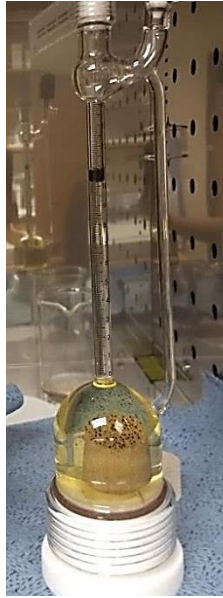
Figure 1.8. Typical oil recoveries through spontaneous imbibition in the presence of surfactants. In this case, spontaneous imbibition is gravity-driven and hence oil is generated mostly from the top surface of the core.
