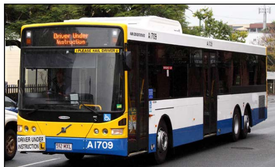
Figure 4-20: 14.5m three axle bus used in Brisbane (base: http://busaustralia.com )
