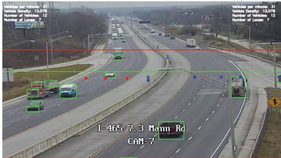
Figure 3.2 Automatically detected lanes and lane direction.
