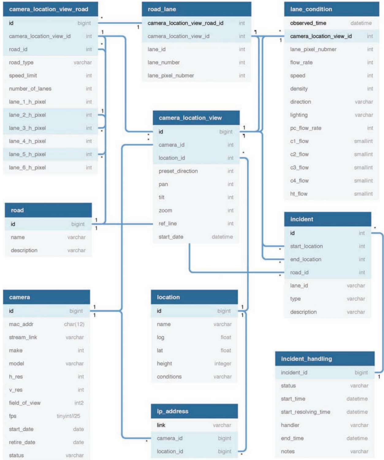
Figure 4.1 ER-diagram of the designed database.
