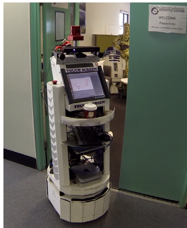
Fig. 1: Our robot after reaching its coffee delivery goal. The robot, like a delivery person, started in an unfamiliar environment and used observed symbolic information to guide itself toward the room that ordered the coffee.
