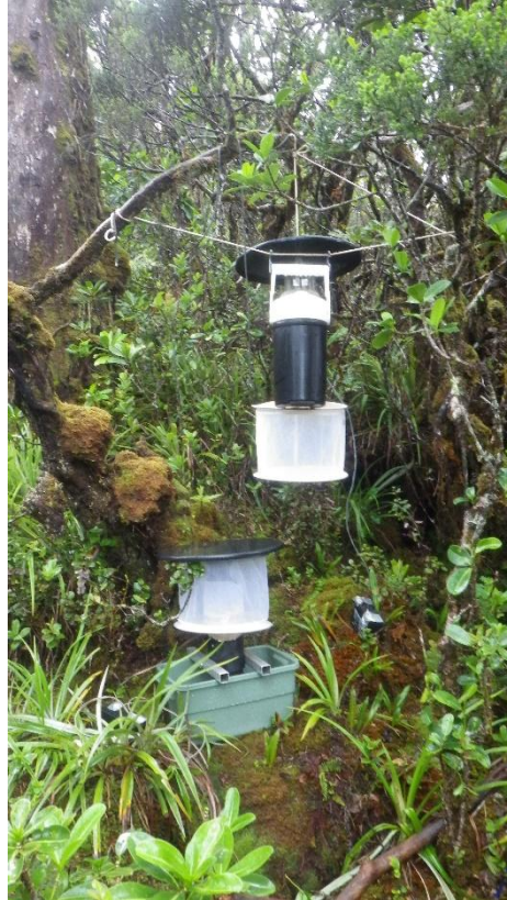
Figure 2. Adult mosquito trap set up showing the CDCP oviposition (on ground) and CDCP light “CO 2 ” (hanging) trap designs.
