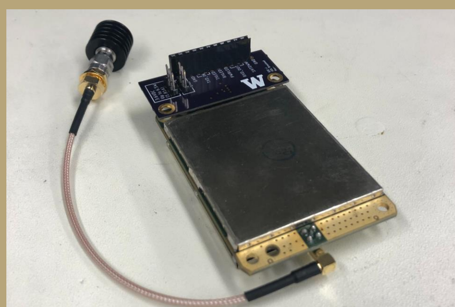
The Pacific Crest XDL Micro radio is being tested at UW currently.
