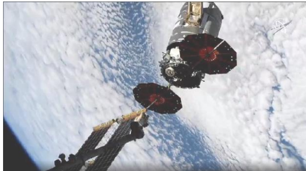
Figure 4: Cygnus NG-12 being Released to Deploy both CubeSats before Reentry
