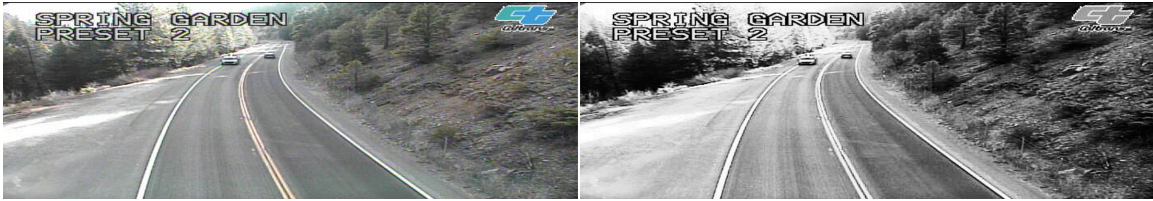
Fig. 4.4: RGB image on left and equivalent histogram equalized image on right.
