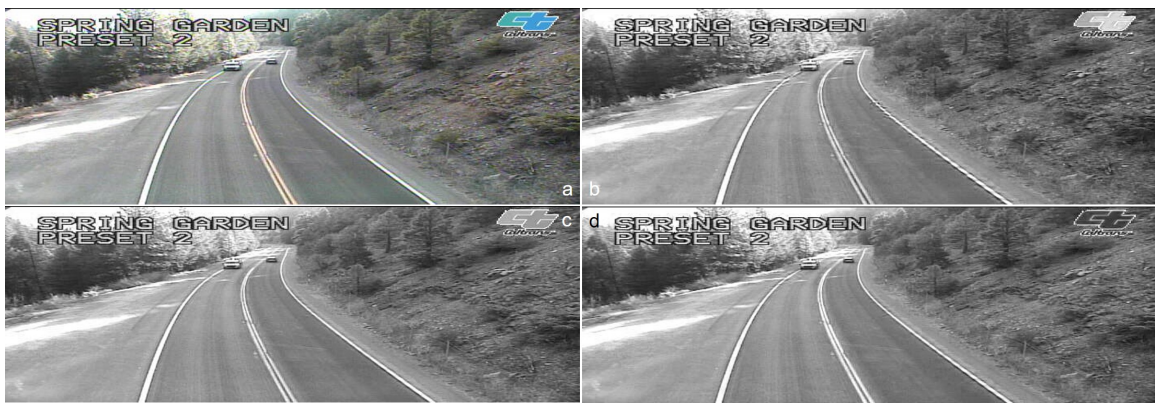
Fig. 4.1: RGB image and its' channels. a, b, c and d indicate all RGB channel, red channel, green channel and blue channel image respectively.
