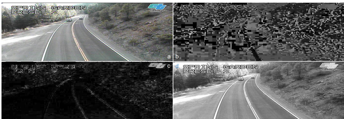
Fig. 4.2: HSV image and its' channels. a, b, c and d indicate all HSV channel, hue channel, saturation channel and variance channel image respectively.
